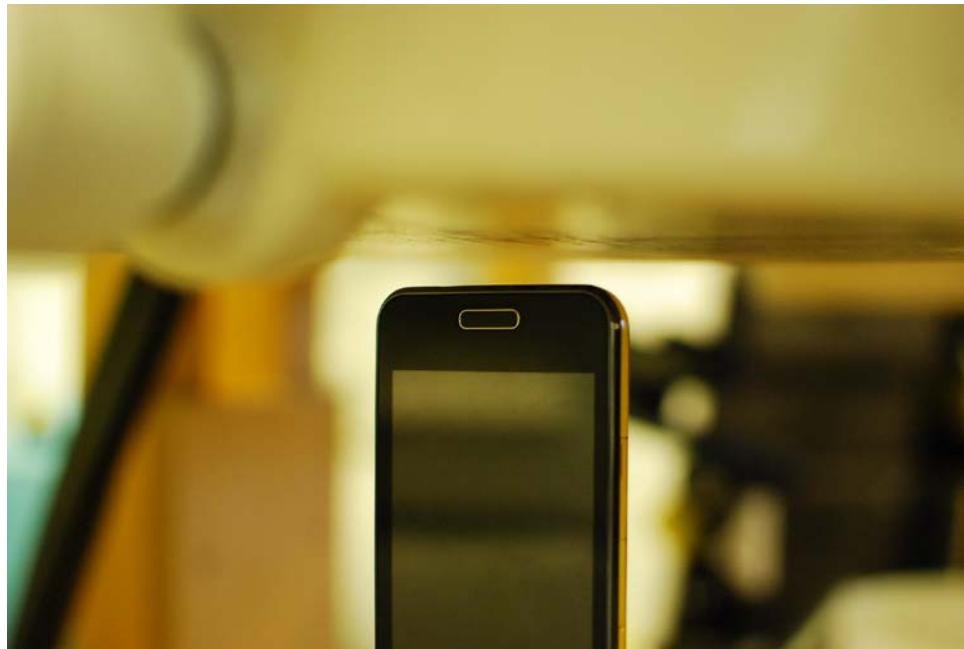
SAR Test Setup Photo 8 – Bottom at 1.0 cm
