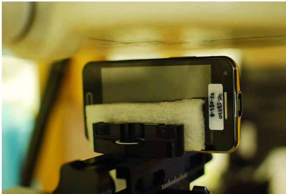
SAR Test Setup Photo 10 – Left at 1.0 cm
