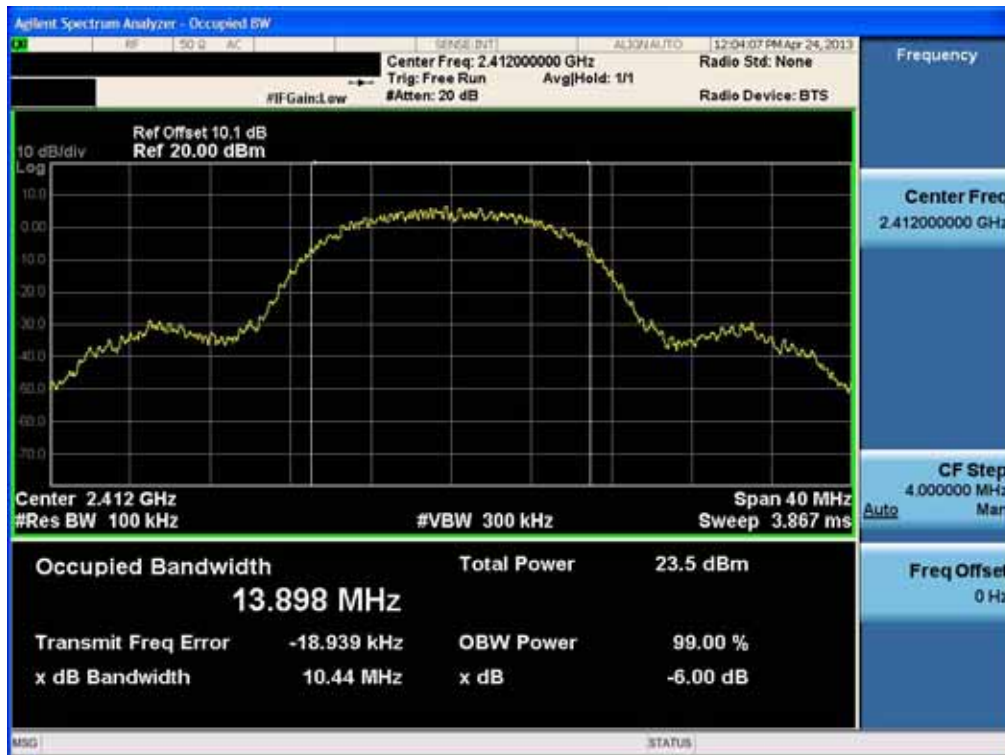
6dB Bandwidth plot (802.11b-CH 6)
