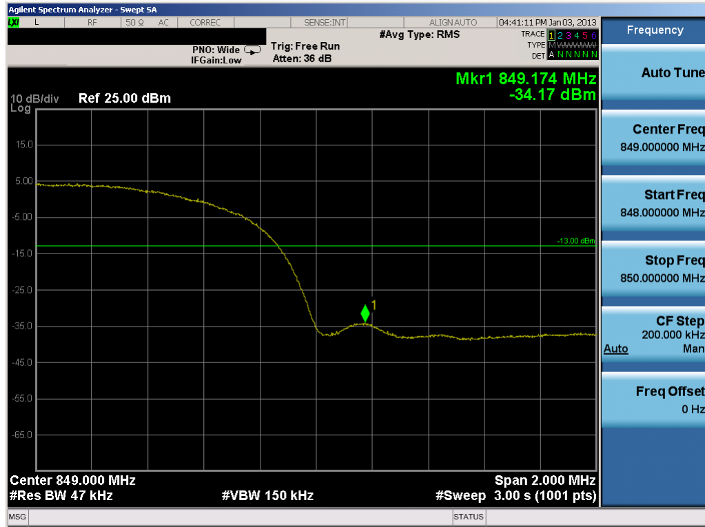
Plot 7-38. Band Edge Plot (Cellular WCDMA Mode – Ch. 4233)
