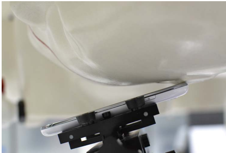
SAR Test Setup Photo 4: Left Tilt
