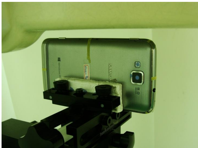
Right Side with Phantom 1 cm Gap
