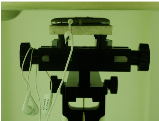
Back of the DUT with Phantom 1 cm Gap (with Headset)
