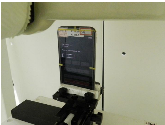
Top Side with Phantom 1 cm Gap
