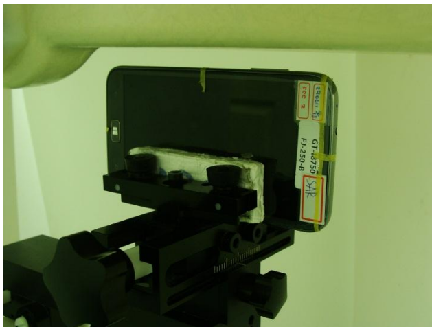
Left Side with Phantom 1 cm Gap
