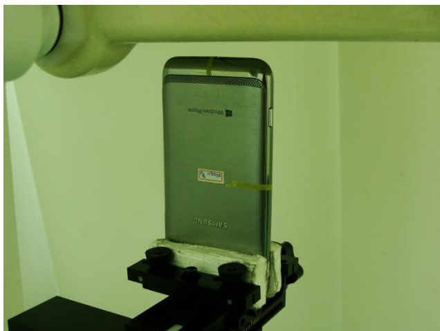
Bottom Side with Phantom 1 cm Gap
