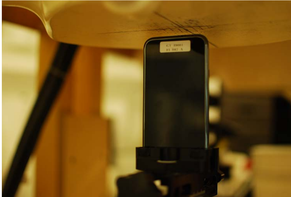
Figure 21-7 SAR Test Setup Photo 7: Top at 1.0 cm
