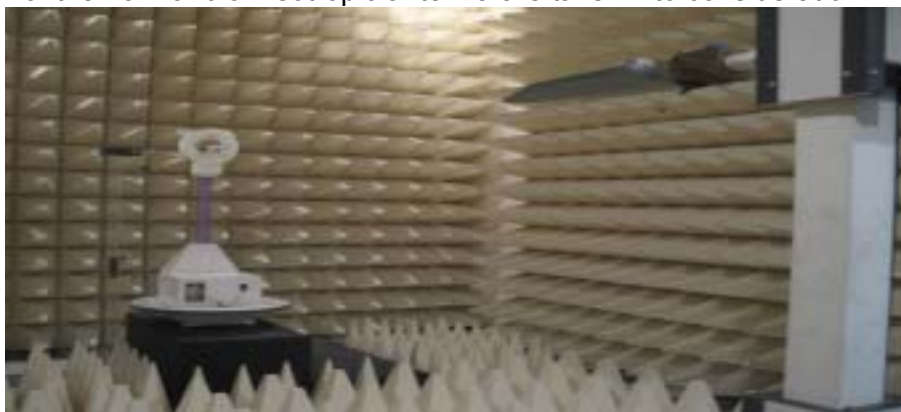
Figure2. Photograph of 3m Fully-Anechoic Chamber
