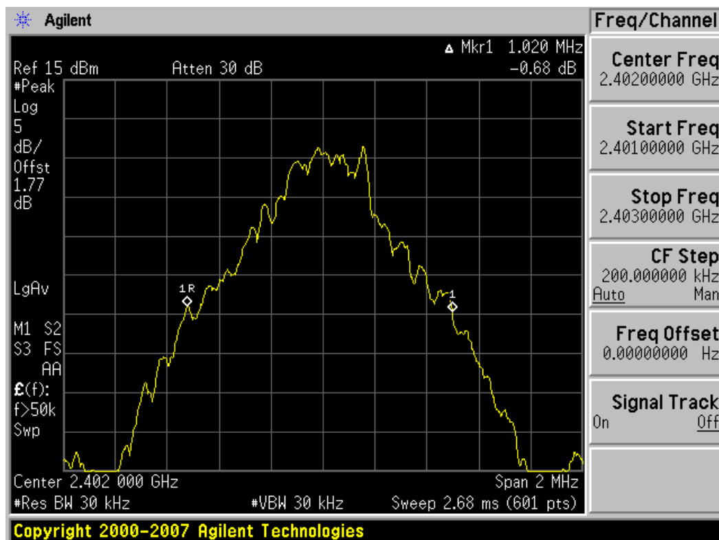
Plot 6-1. 20dB Bandwidth Plot (Bluetooth, 1Mbps – Ch. 0)
