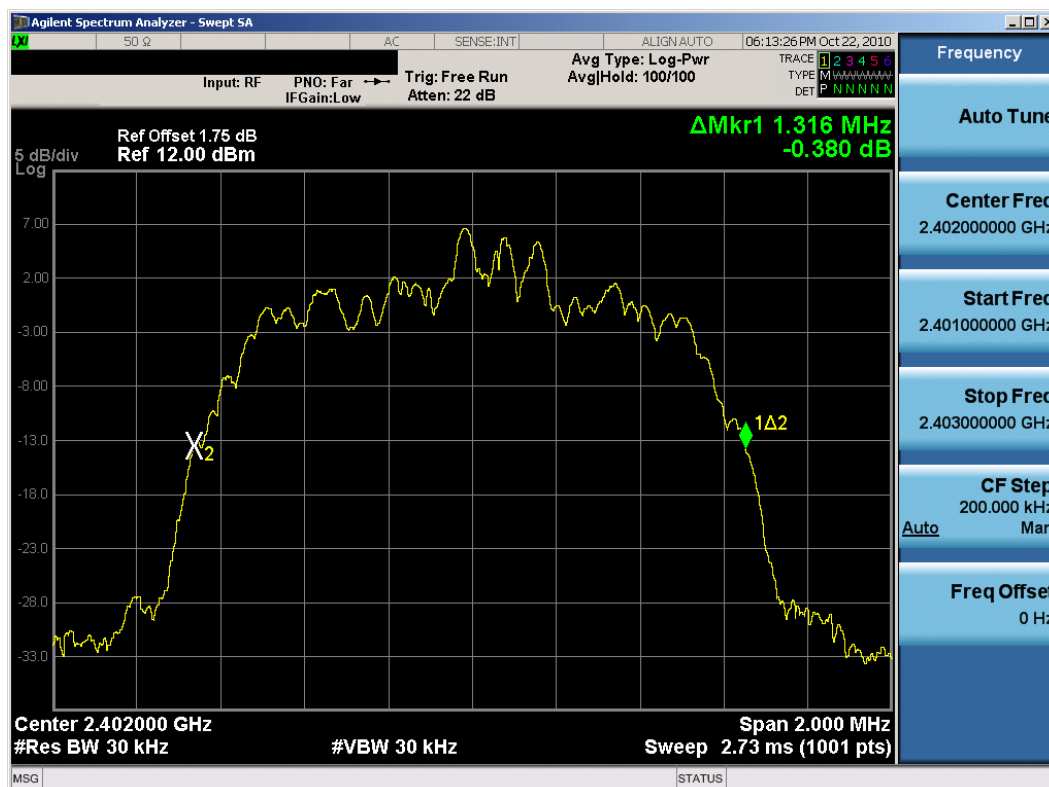
Plot 6-4. 20dB Bandwidth Plot (Bluetooth, 2Mbps – Ch. 0)
