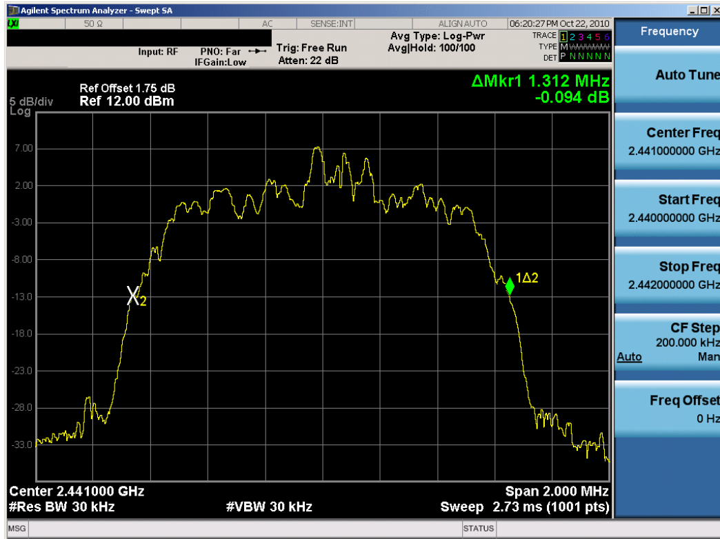
Plot 6-5. 20dB Bandwidth Plot (Bluetooth, 2Mbps – Ch. 39)
