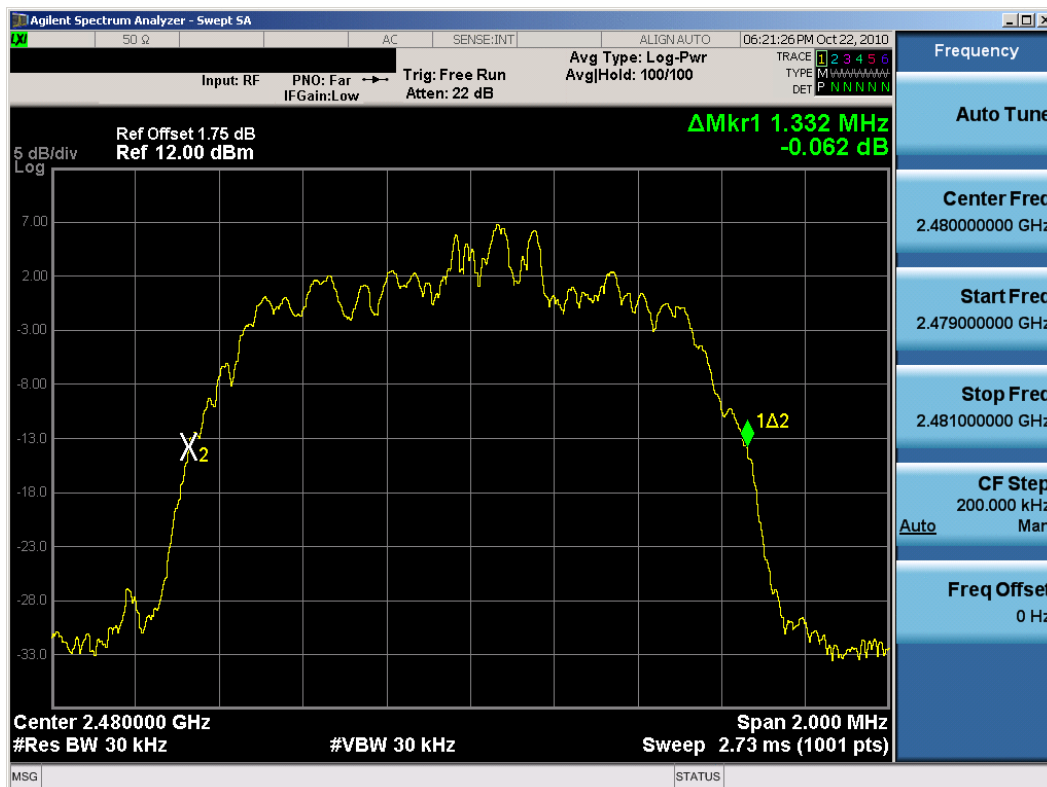
Plot 6-6. 20dB Bandwidth Plot (Bluetooth, 2Mbps – Ch. 78)
