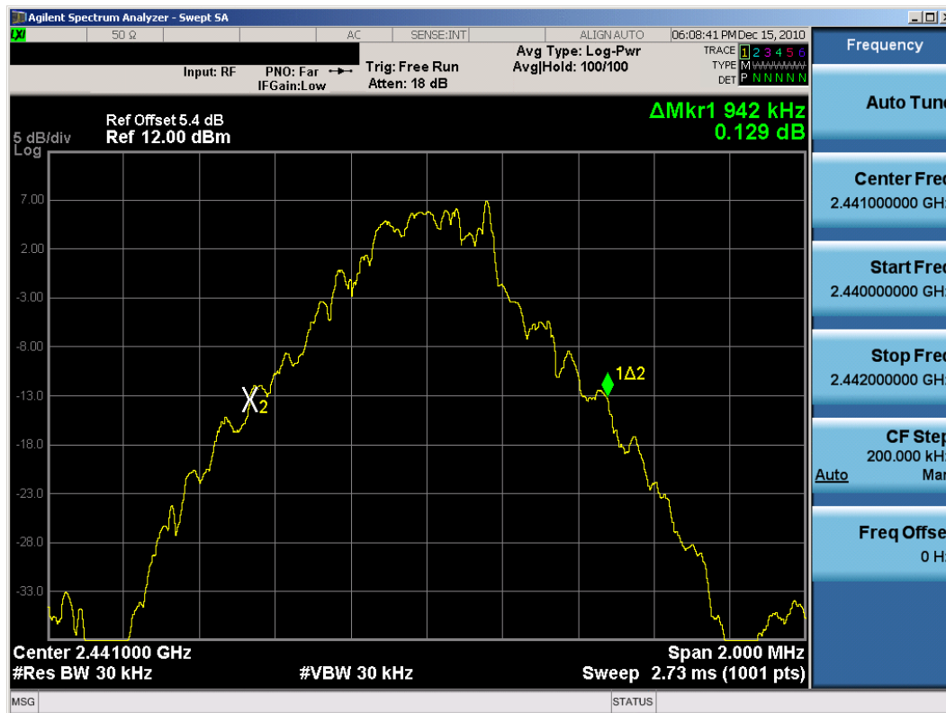
Plot 6-2. 20dB Bandwidth Plot (Bluetooth, 1Mbps - Ch. 39)
