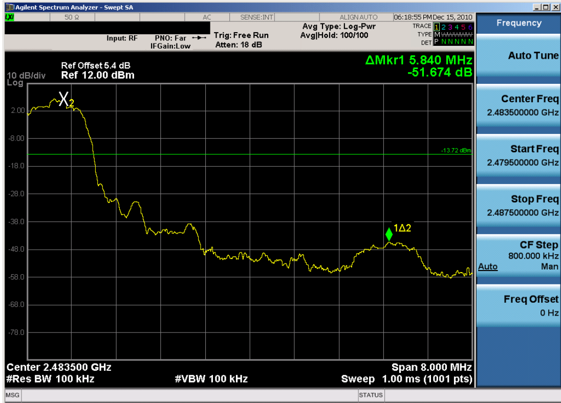
Plot 6-13. Band Edge Plot (Bluetooth, 3Mbps – Ch. 78)
