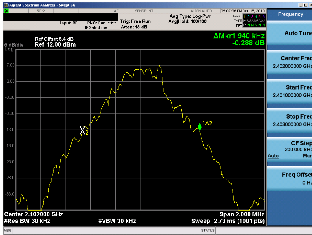
Plot 6-1. 20dB Bandwidth Plot (Bluetooth, 1Mbps - Ch. 0)
