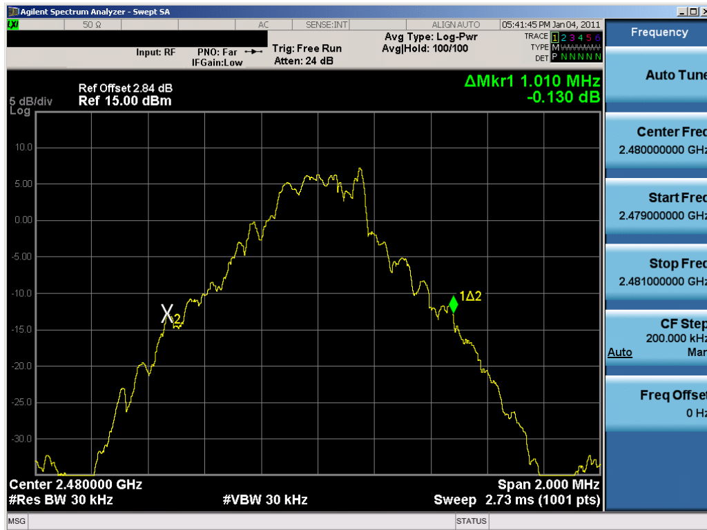
Plot 6-3. 20dB Bandwidth Plot (Bluetooth, 1Mbps – Ch. 78)
