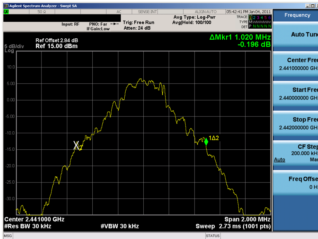
Plot 6-2. 20dB Bandwidth Plot (Bluetooth, 1Mbps - Ch. 39)
