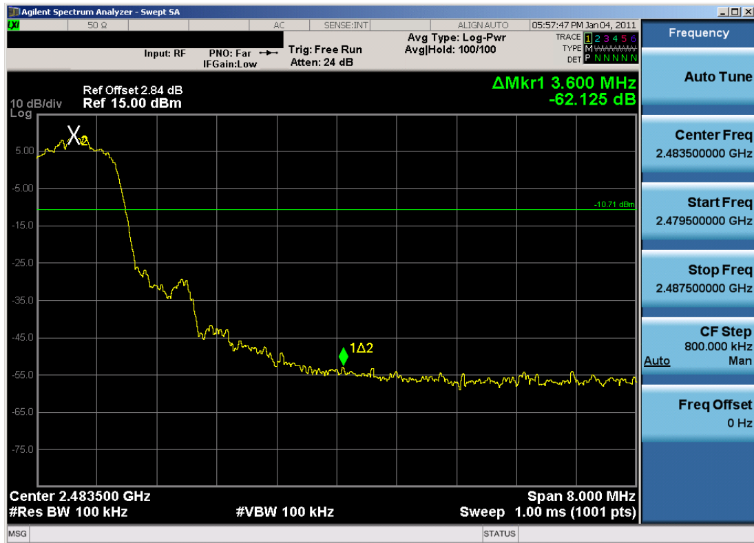
Plot 6-13. Band Edge Plot (Bluetooth, 2Mbps – Ch. 78)
