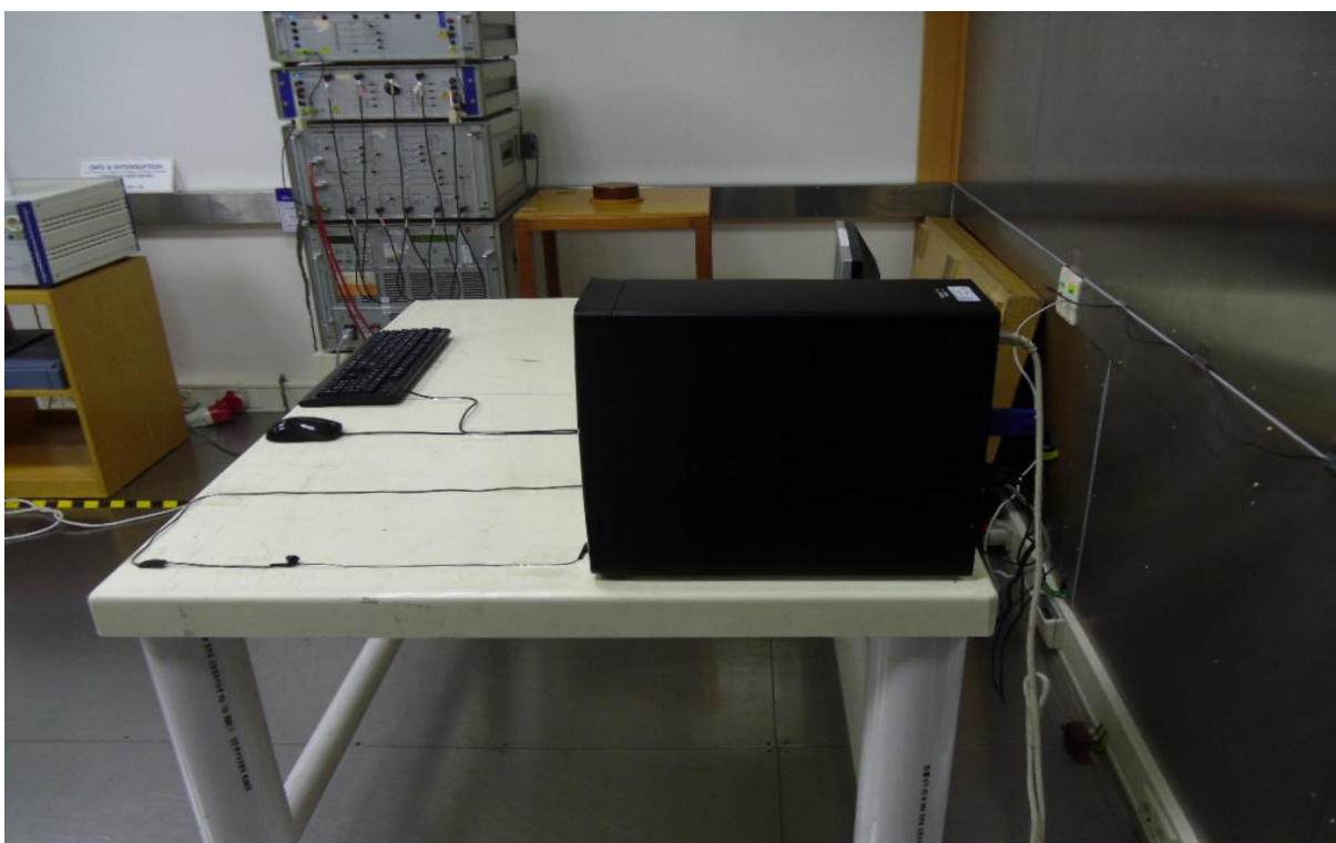
[ Conducted Disturbance – Rear ]
