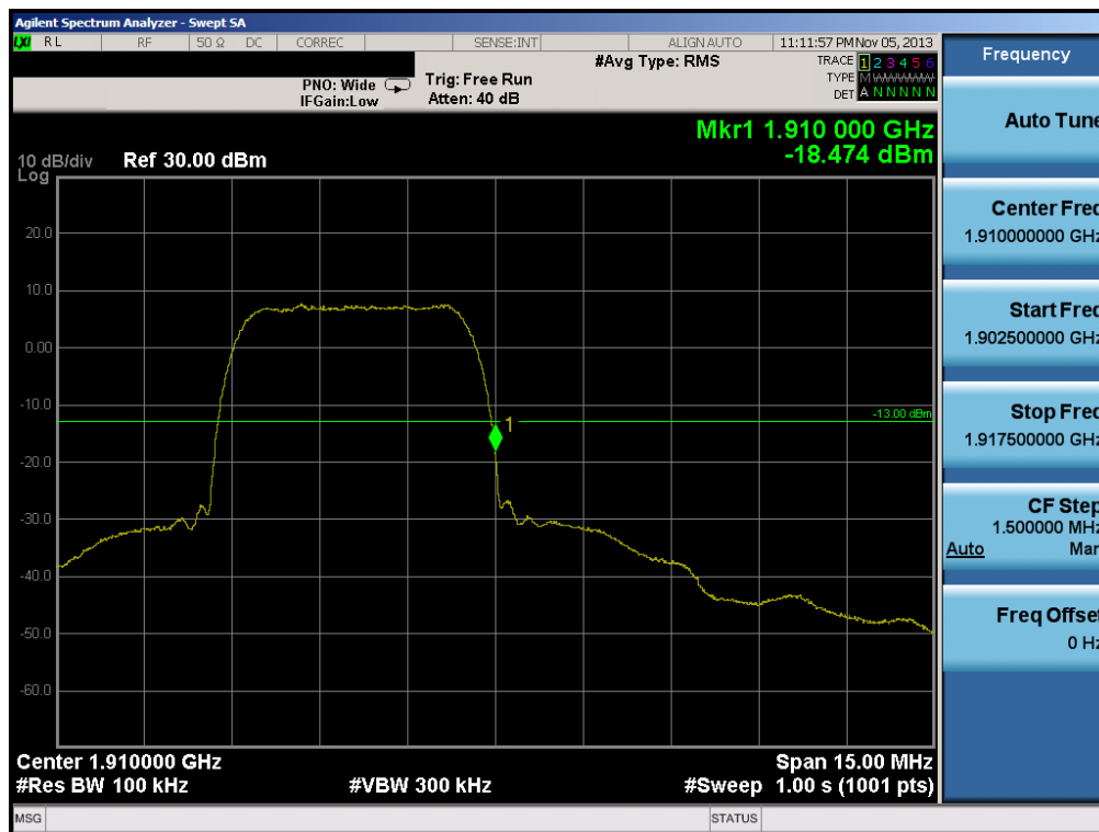
Plot 6-31. Band Edge Plot (PCS WCDMA Mode – Ch. 9538)
