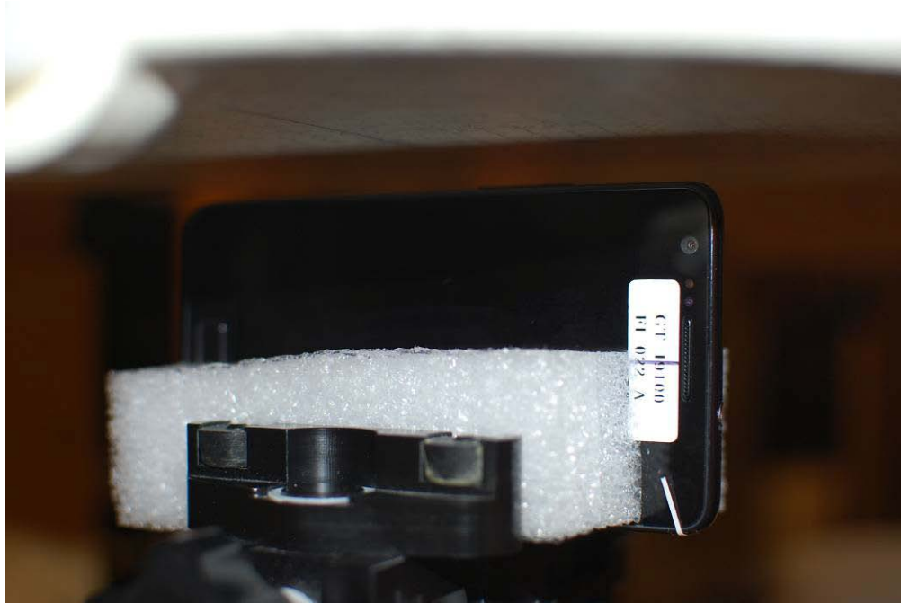
Figure 21-9 SAR Test Photo 9– Left at 1.0 cm
