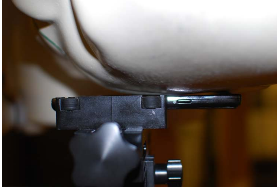
SAR Test Setup Photo 3: Left Touch
