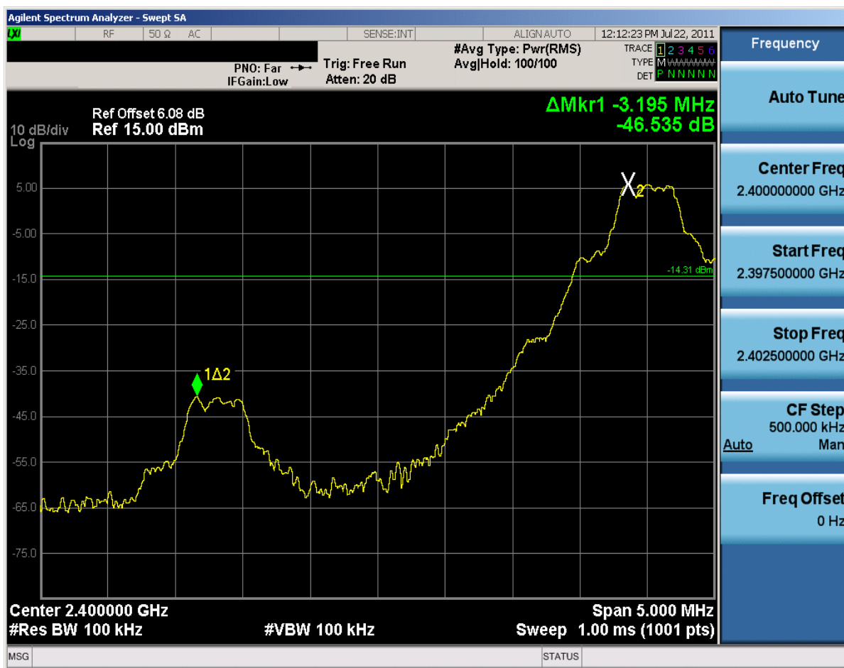
Plot 6-10. Band Edge Plot (Bluetooth, 1Mbps – Ch. 0)
