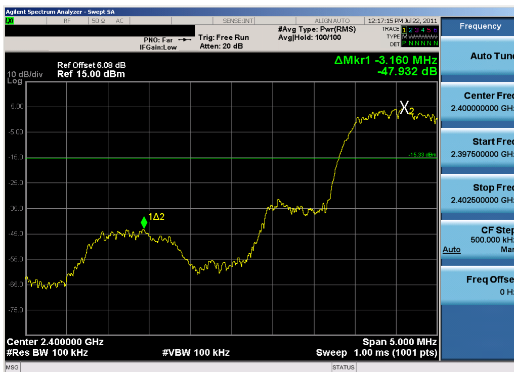
Plot 6-12. Band Edge Plot (Bluetooth, 3Mbps – Ch. 0)
