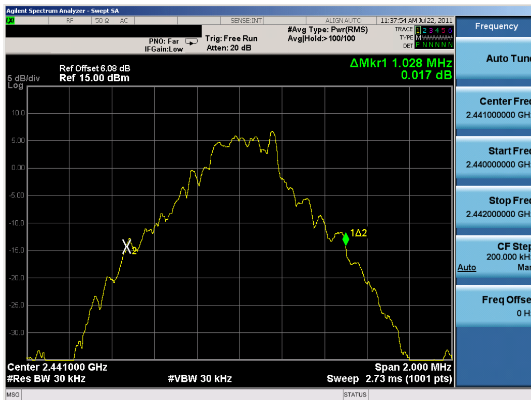
Plot 6-2. 20dB Bandwidth Plot (Bluetooth, 1Mbps – Ch. 39)
