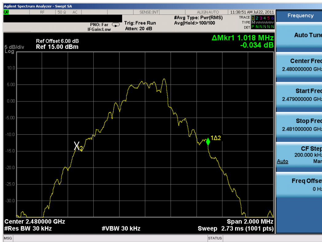
Plot 6-3. 20dB Bandwidth Plot (Bluetooth, 1Mbps – Ch. 78)
