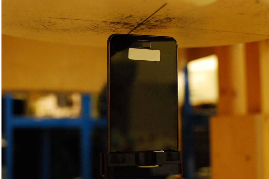
SAR Test Setup Photo 7 – Bottom at 1.0 cm
