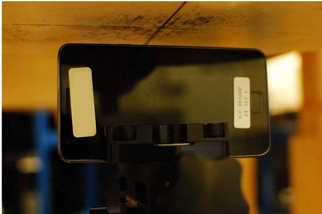
SAR Test Setup Photo 8 – Right at 1.0 cm
