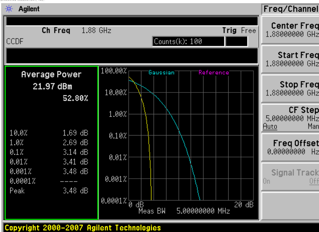
Plot 7-41. Peak-Average Ratio Plot (PCS WCDMA Mode – Ch. 9400)
