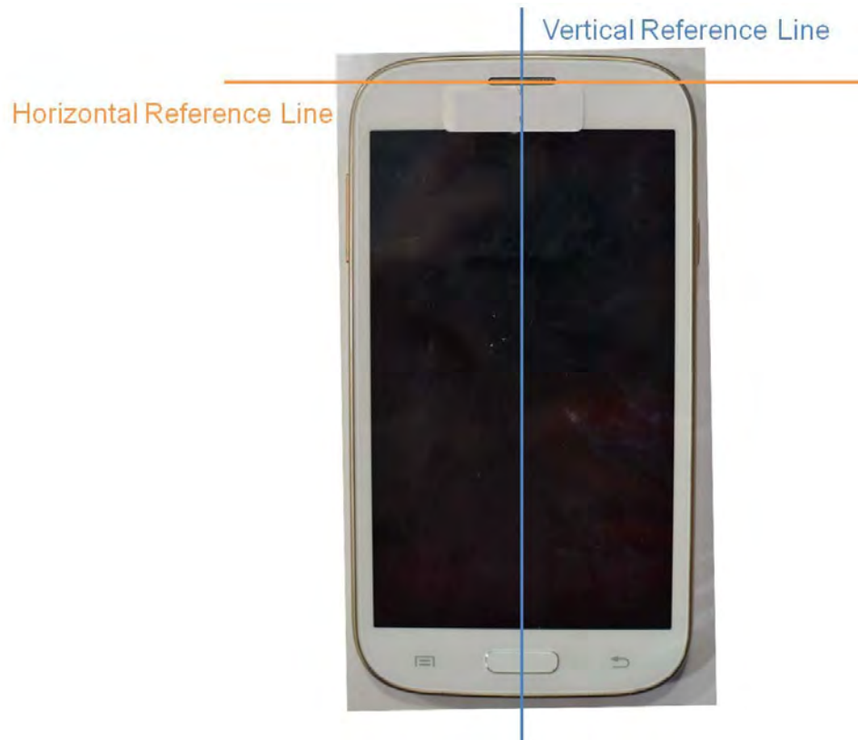
SAR Test Setup Photo 10 – Horizontal and Vertical Reference Lines
