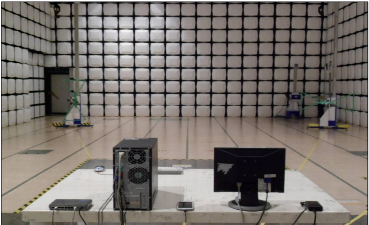
[ Radiated Disturbance for Below 1 GHz – Rear ]
