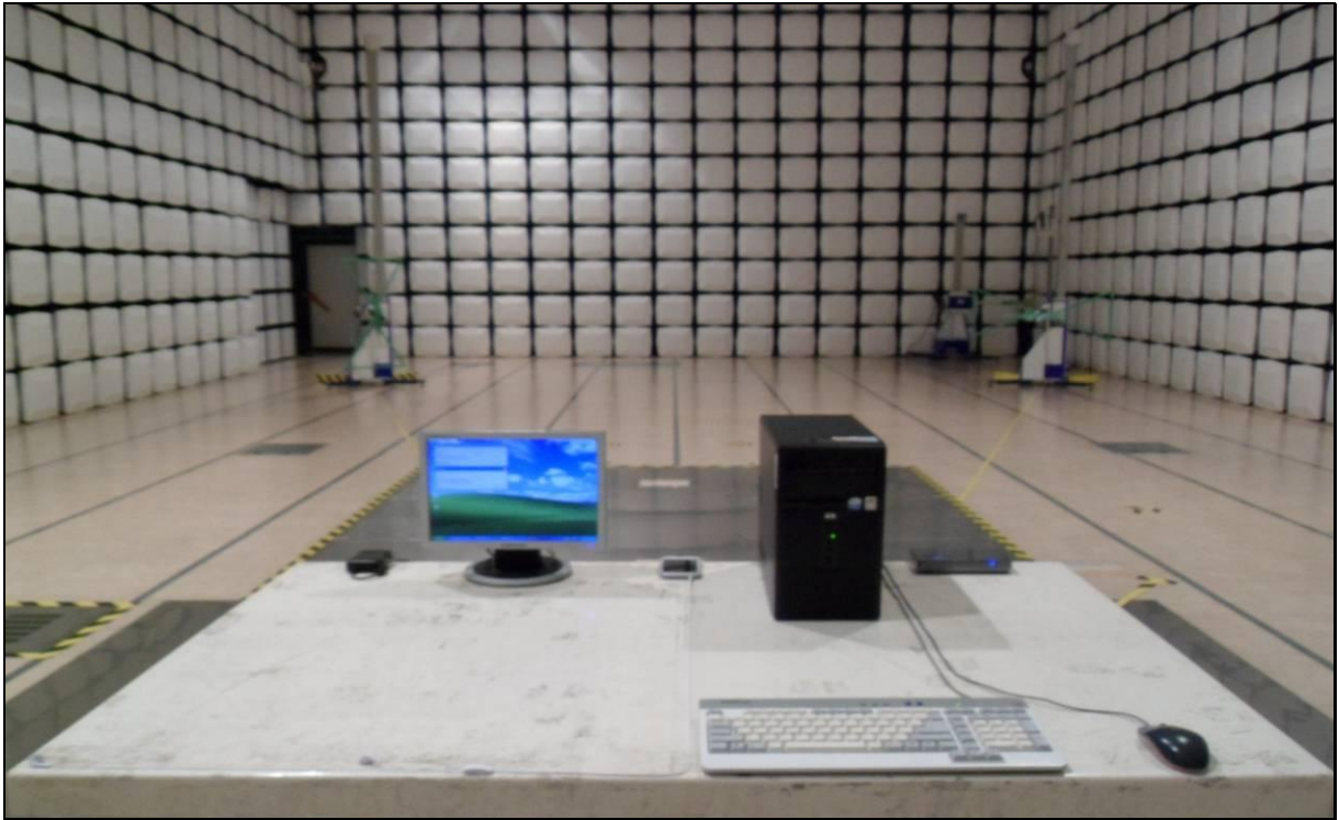
[ Radiated Disturbance for Below 1 GHz – Front ]
