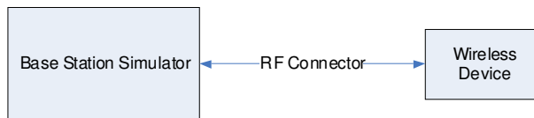
Figure 8-1 Power Measurement Setup
