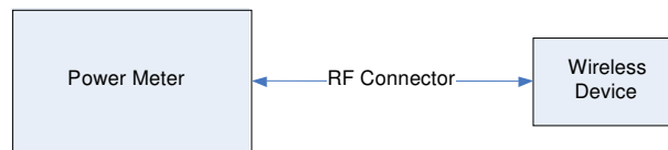
Figure 8-3 Power Measurement Setup
