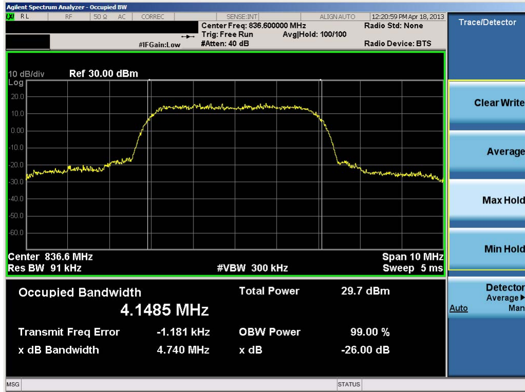
Plot 7-28. Occupied Bandwidth Plot (Cellular WCDMA Mode – Ch. 4183)
