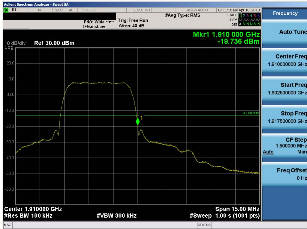
Plot 7-42. Band Edge Plot (PCS WCDMA Mode – Ch. 9538)
