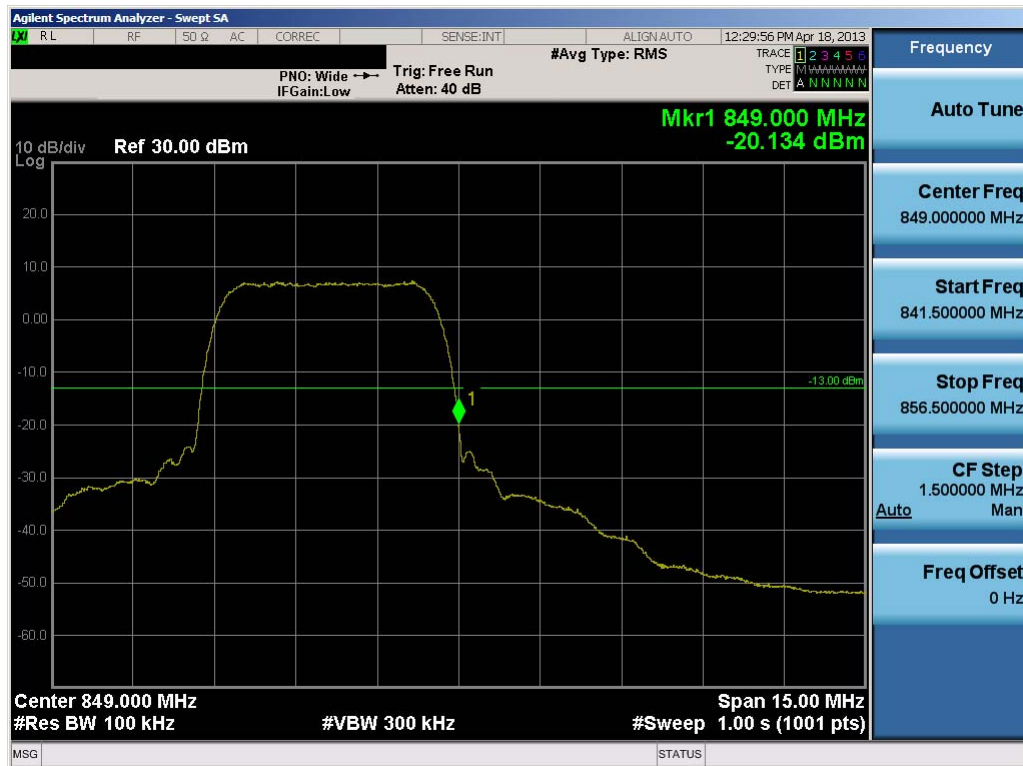
Plot 7-31. Band Edge Plot (Cellular WCDMA Mode – Ch. 4233)
