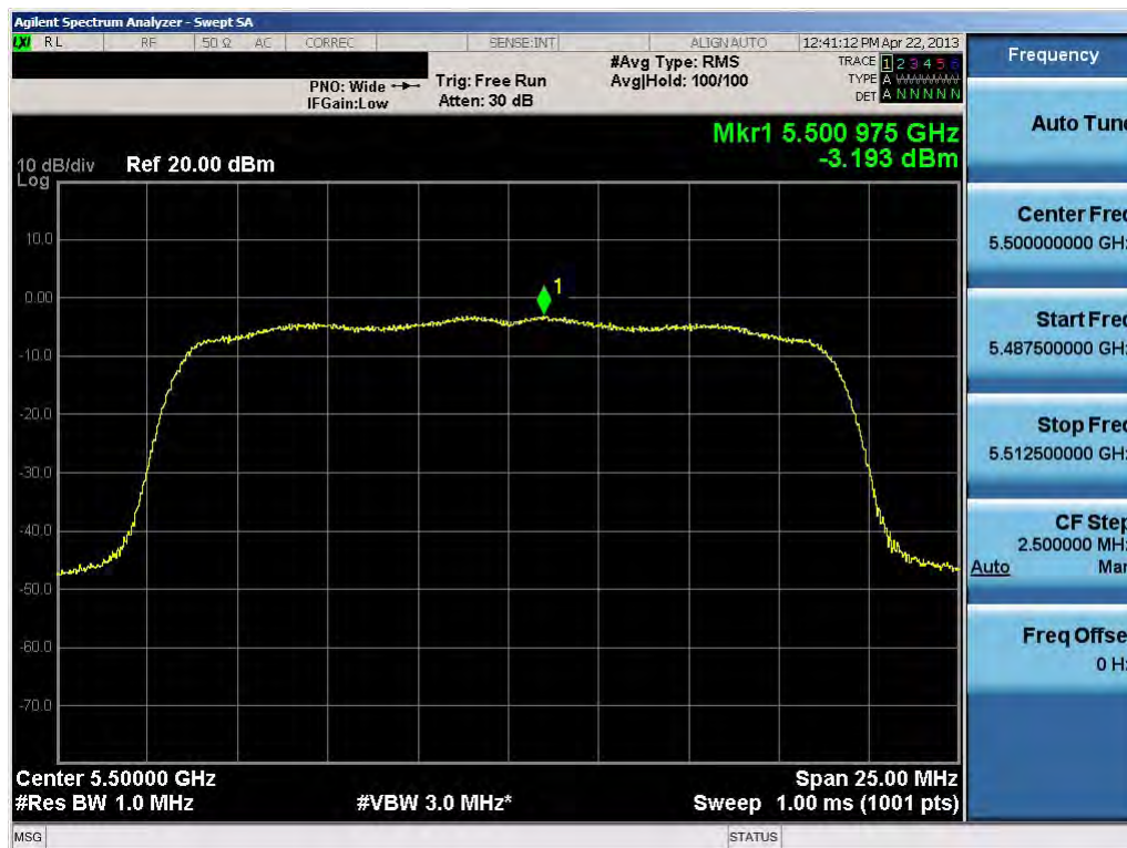
Plot 6-45. Peak Power Spectral Density Plot (20MHz BW 802.11n (UNII Band 3) – Ch. 100)
