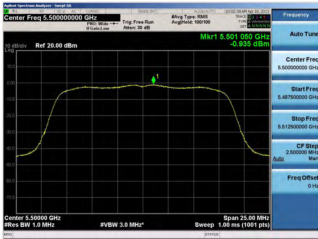
Plot 6-42. Peak Power Spectral Density Plot (802.11a (UNII Band 3) - Ch. 100)
