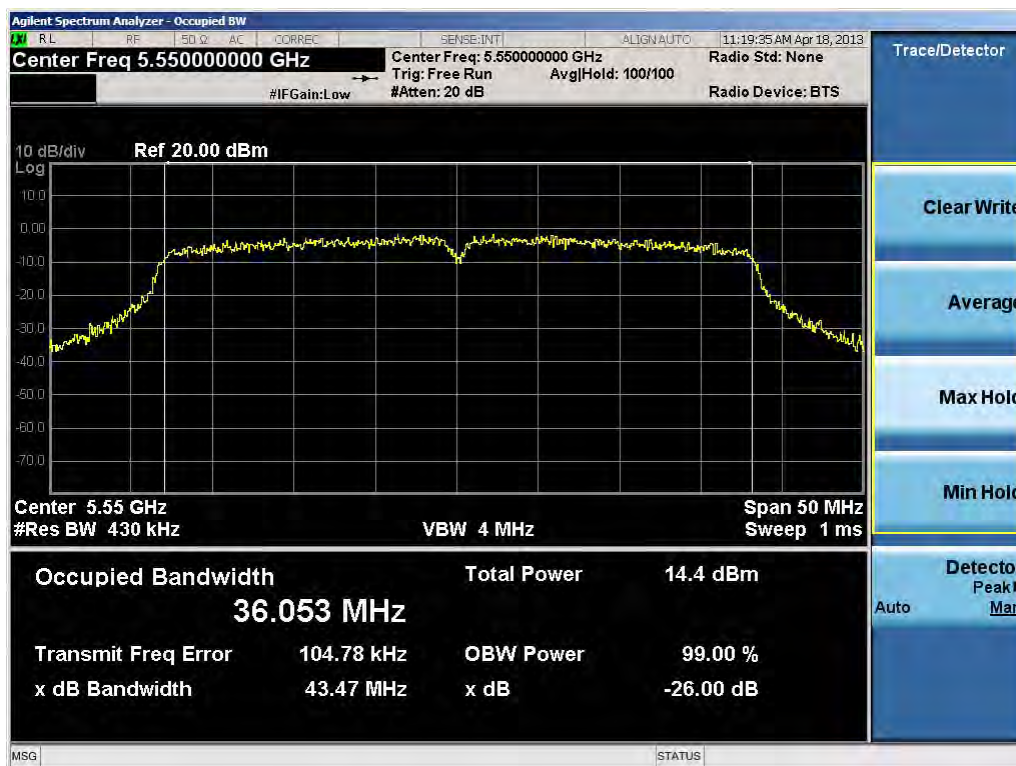
Plot 6-24. 26dB Bandwidth Plot (40MHz BW 802.11n (UNII Band 3) – Ch. 110)
