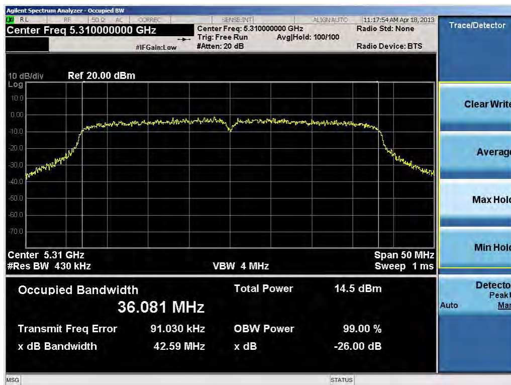
Plot 6-16. 26dB Bandwidth Plot (40MHz BW 802.11n (UNII Band 2) – Ch. 62)
