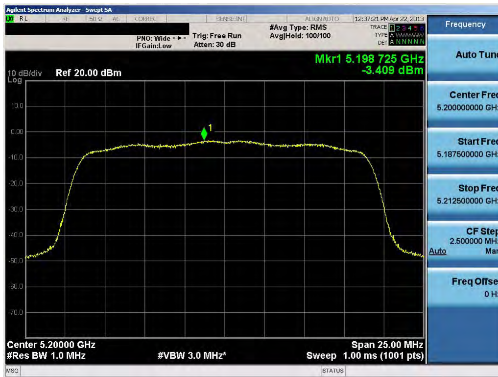
Plot 6-30. Peak Power Spectral Density Plot (20MHz BW 802.11n (UNII Band 1) – Ch. 40)
