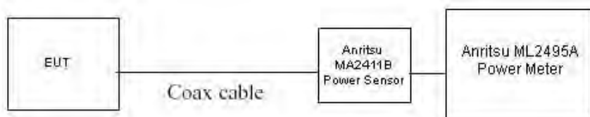
Figure 6-2. Test Instrument & Measurement Setup
