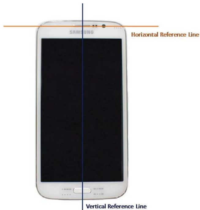
SAR Test Setup Photo 10: Vertical and Horizontal Reference Lines
