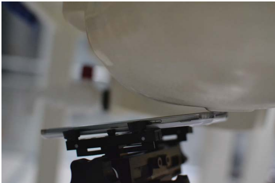
SAR Test Setup Photo 4: Left Tilt
