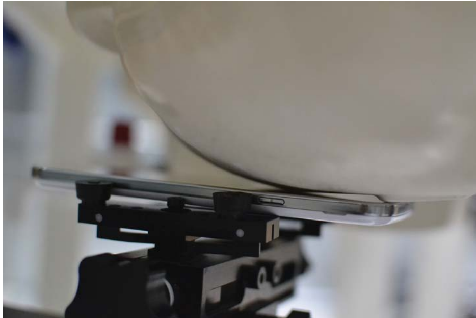
SAR Test Setup Photo 3: Left Cheek
