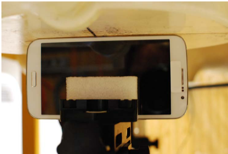
SAR Test Setup Photo 12: Left at 0.0 cm (Hand SAR Testing)
