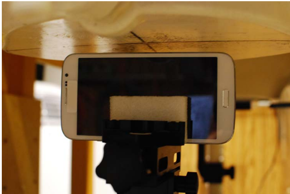
SAR Test Setup Photo 8: Right at 1.0 cm
