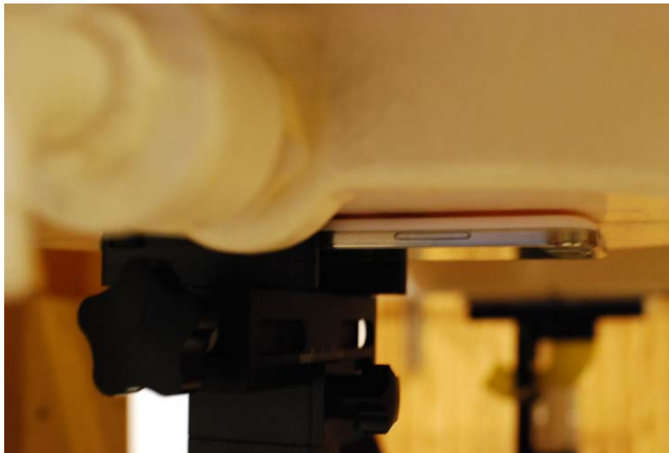
SAR Test Setup Photo 10: Back at 0.0 cm (Hand SAR Testing)
