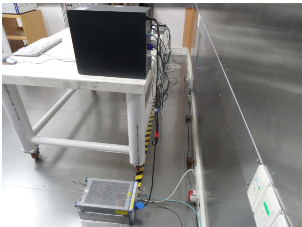
[ Conducted Disturbance – Rear ]
