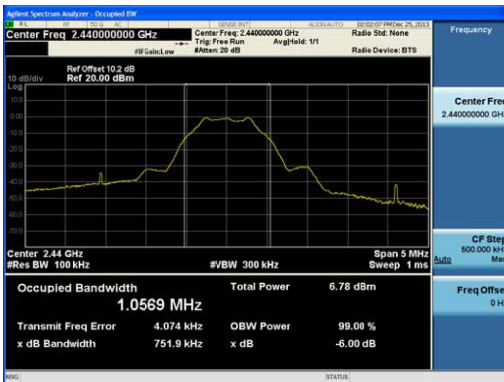
6dB Bandwidth plot (Mid-CH 19)
