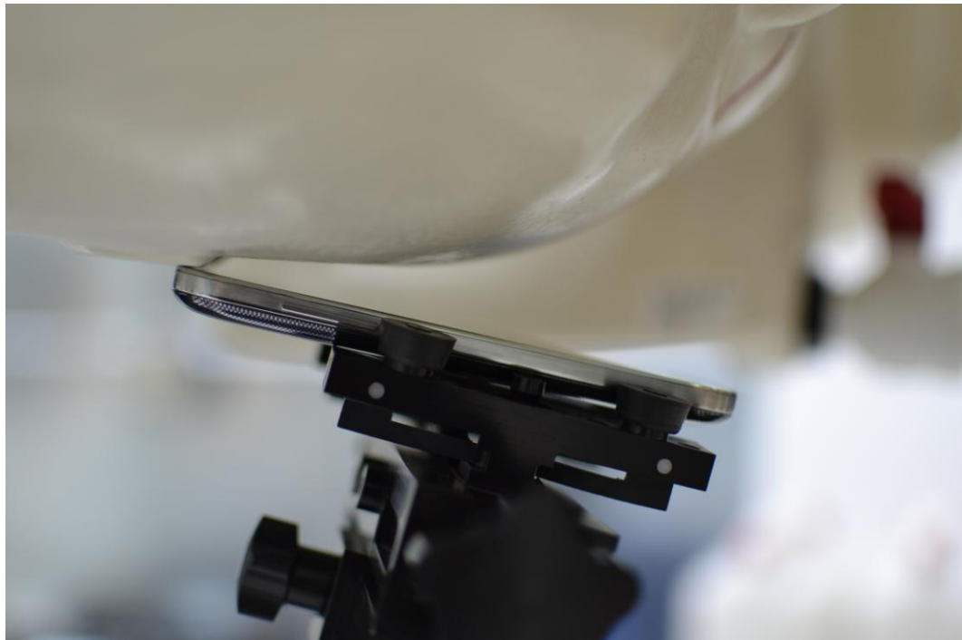
SAR Test Setup Photo 2: Right Tilt
