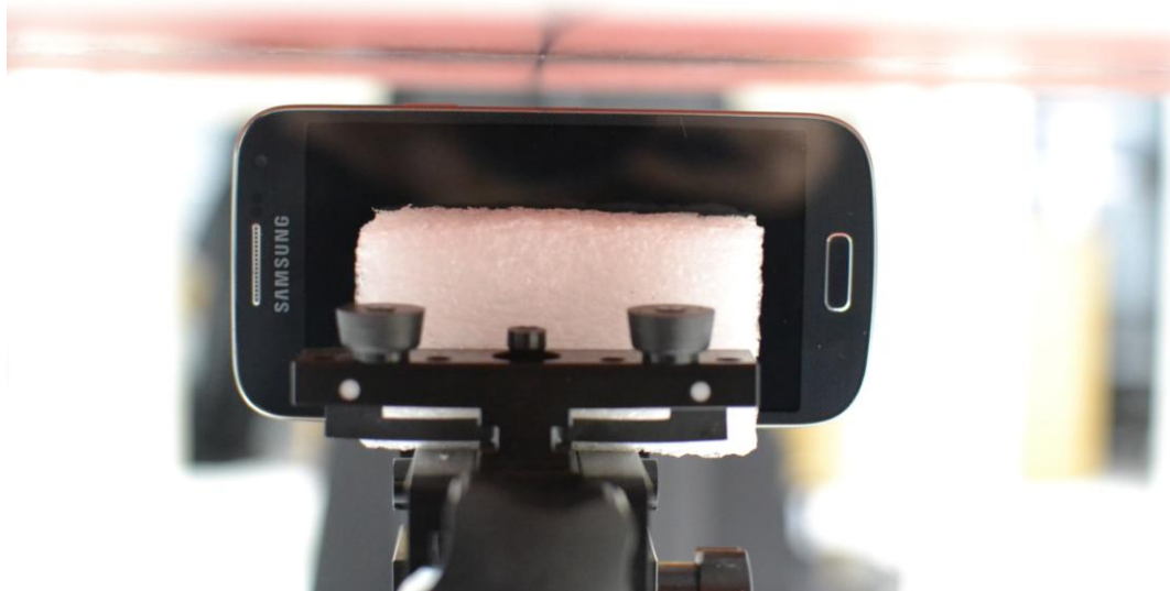
SAR Test Setup Photo 8: Right Edge at 1.0 cm
