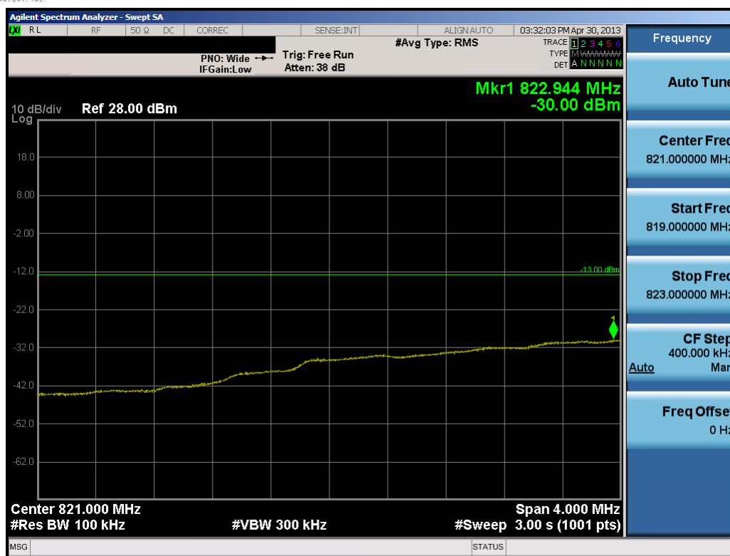
Plot 7-22. Lower Extended Band Edge Plot (5.0MHz QPSK – RB Size 25)
