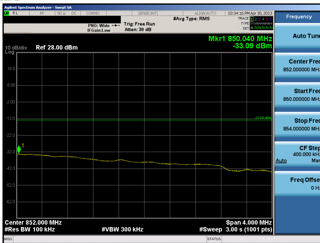
Plot 7-32. Upper Extended Band Edge Plot (5.0MHz QPSK – RB Size 25)
