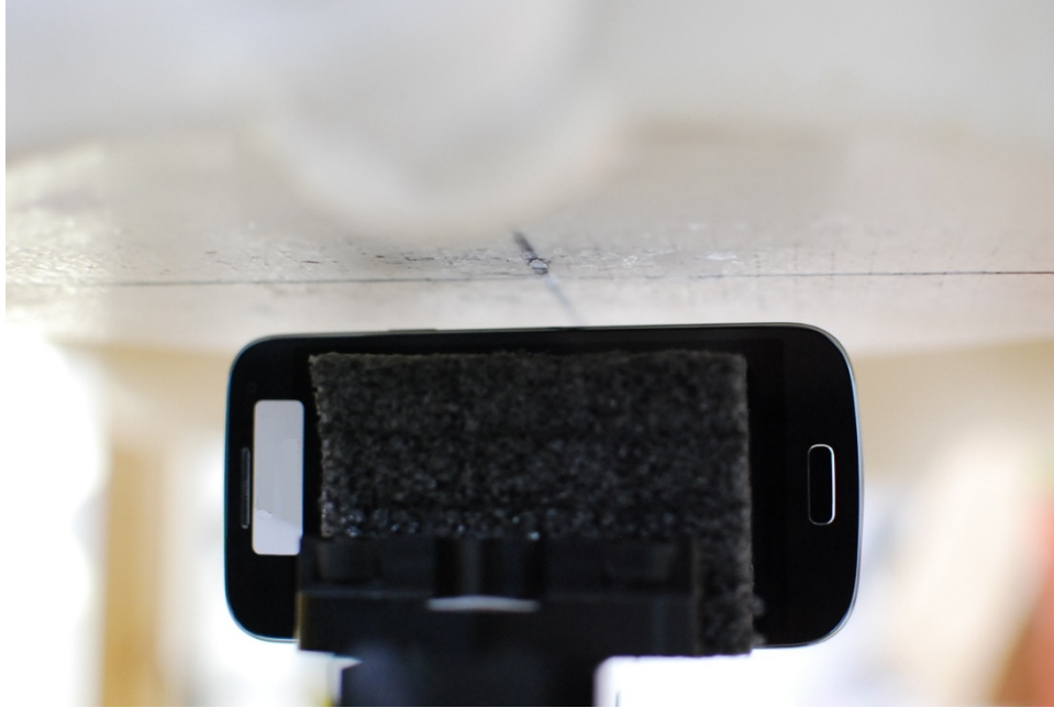
SAR Test Setup Photo 9: Right at 1.0 cm
