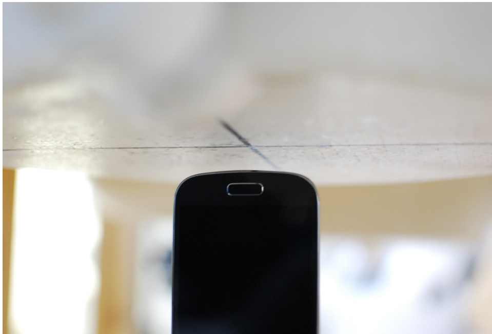
SAR Test Setup Photo 8: Bottom at 1.0 cm
