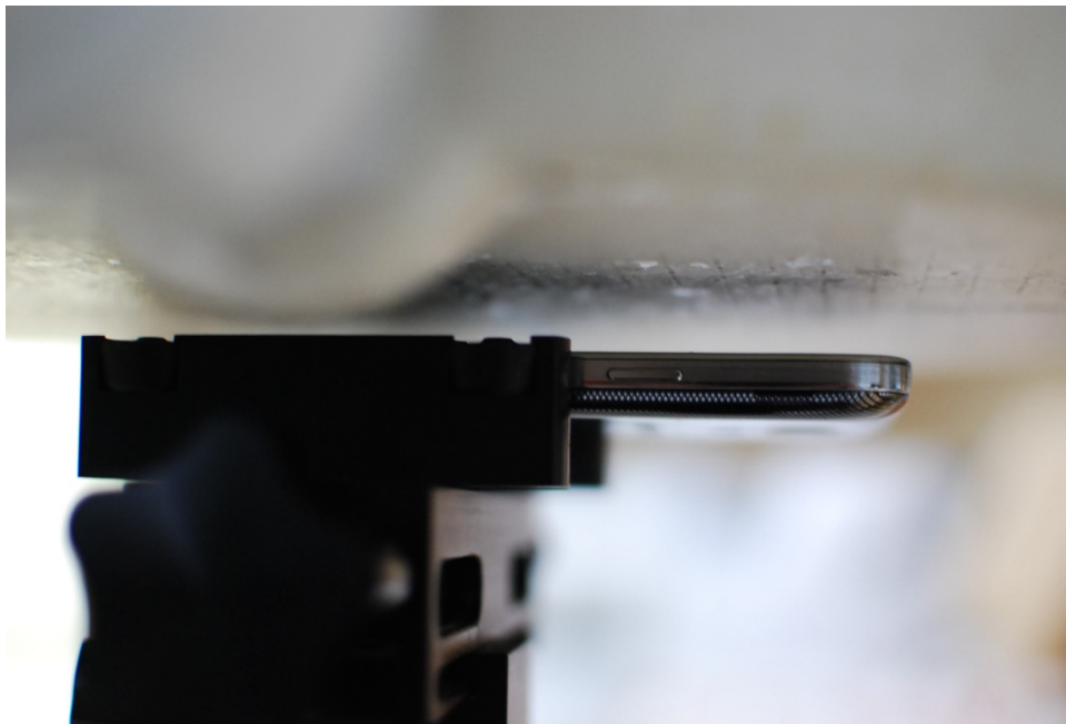
SAR Test Setup Photo 6: Front at 1.0 cm
