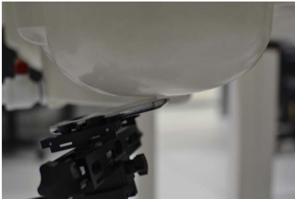
SAR Test Setup Photo 4: Left Tilt
