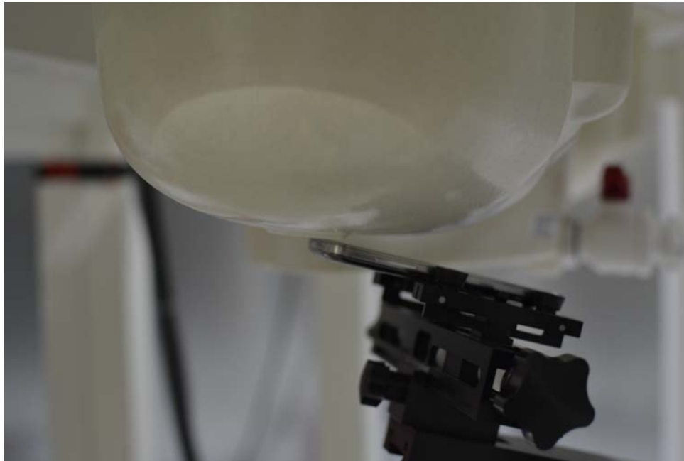
SAR Test Setup Photo 2: Right Tilt
