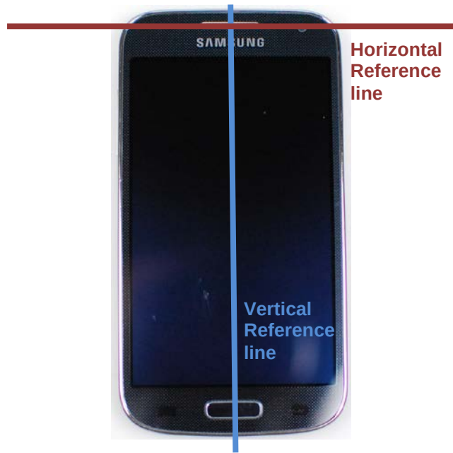
SAR Test Setup Photo 11: DUT Reference Lines
