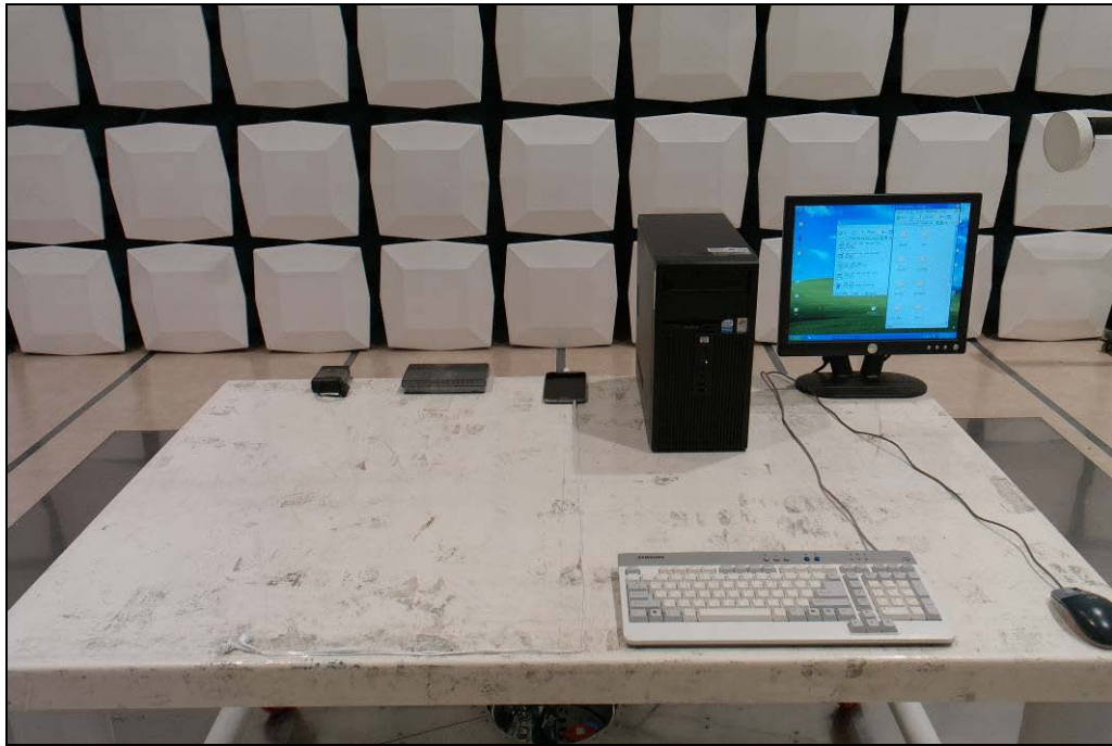
[ Radiated Disturbance for Below 1 GHz – Front ]
