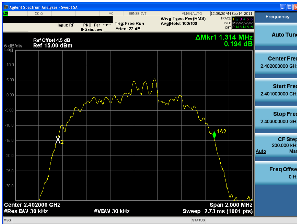
Plot 6-7. 20dB Bandwidth Plot (Bluetooth, 3Mbps – Ch. 0)
