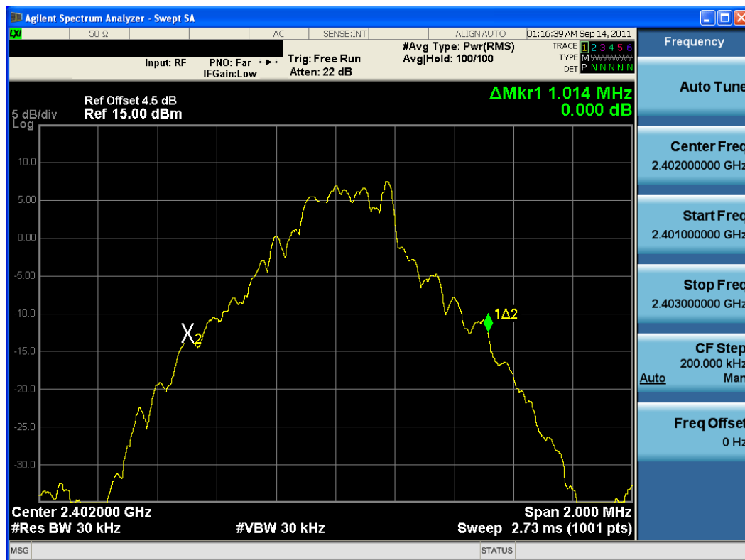
Plot 6-1. 20dB Bandwidth Plot (Bluetooth, 1Mbps – Ch. 0)
