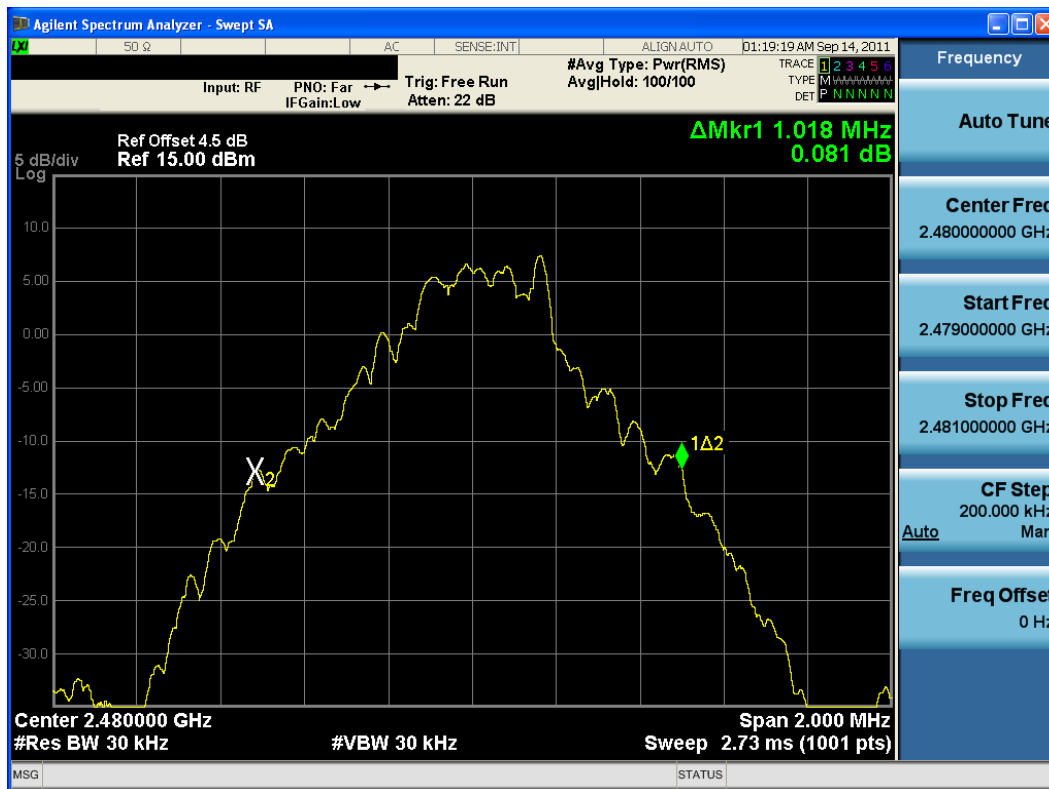
Plot 6-3. 20dB Bandwidth Plot (Bluetooth, 1Mbps – Ch. 78)
