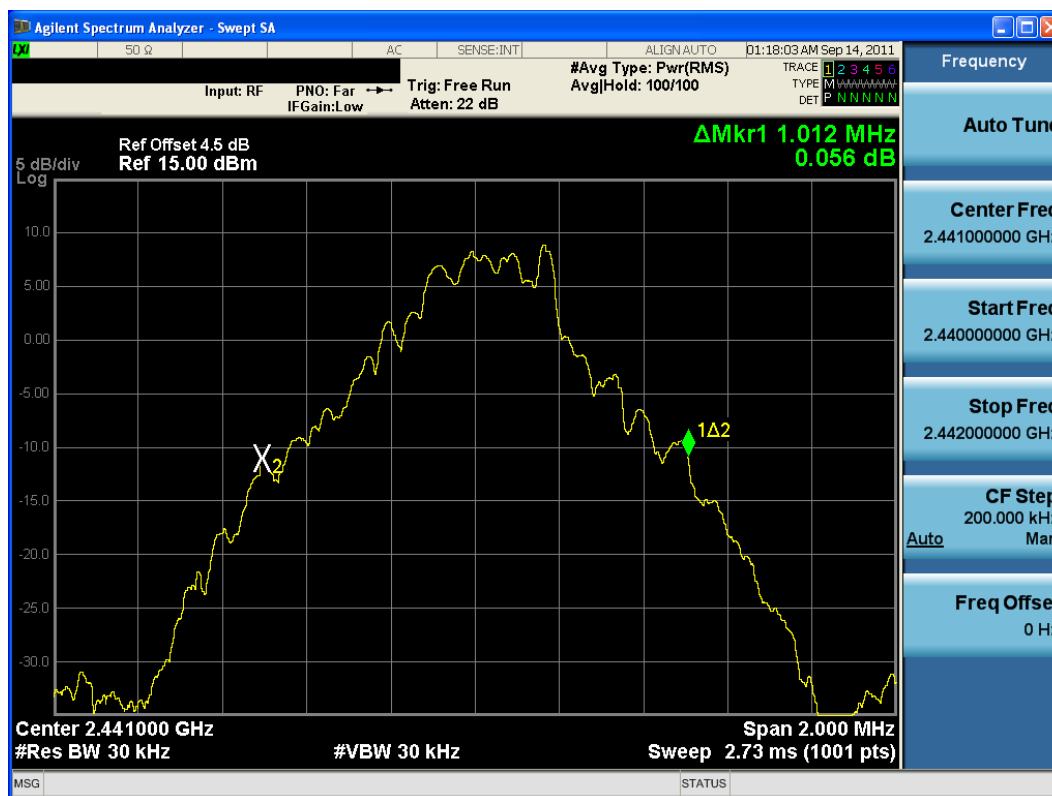
Plot 6-2. 20dB Bandwidth Plot (Bluetooth, 1Mbps – Ch. 39)
