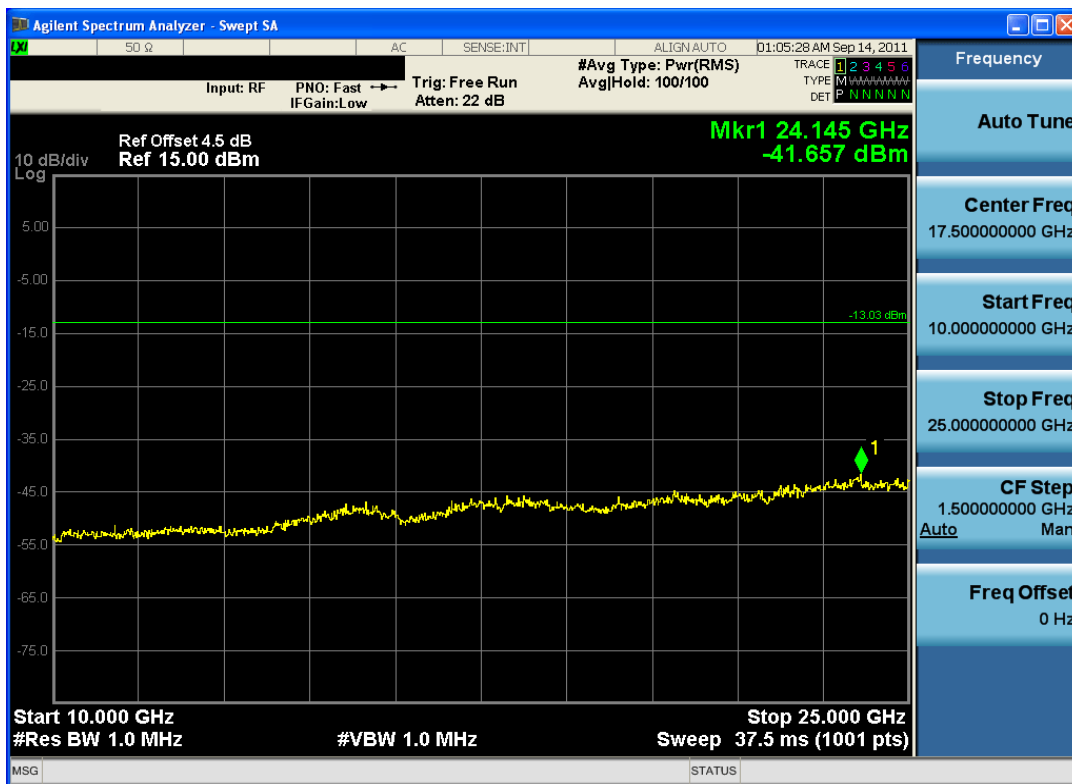
Plot 6-21. Conducted Spurious Plot (Bluetooth, 3Mbps – Ch. 78)
