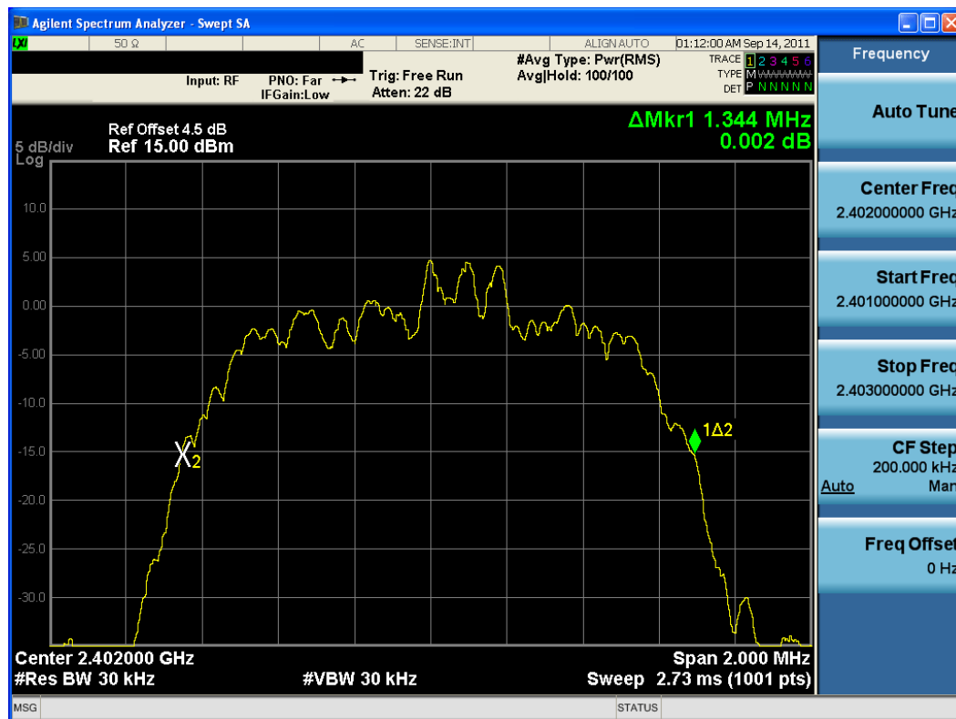
Plot 6-4. 20dB Bandwidth Plot (Bluetooth, 2Mbps – Ch. 0)
