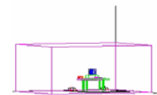
Figure 3-1. Shielded Enclosure Line-Conducted Test Facility
