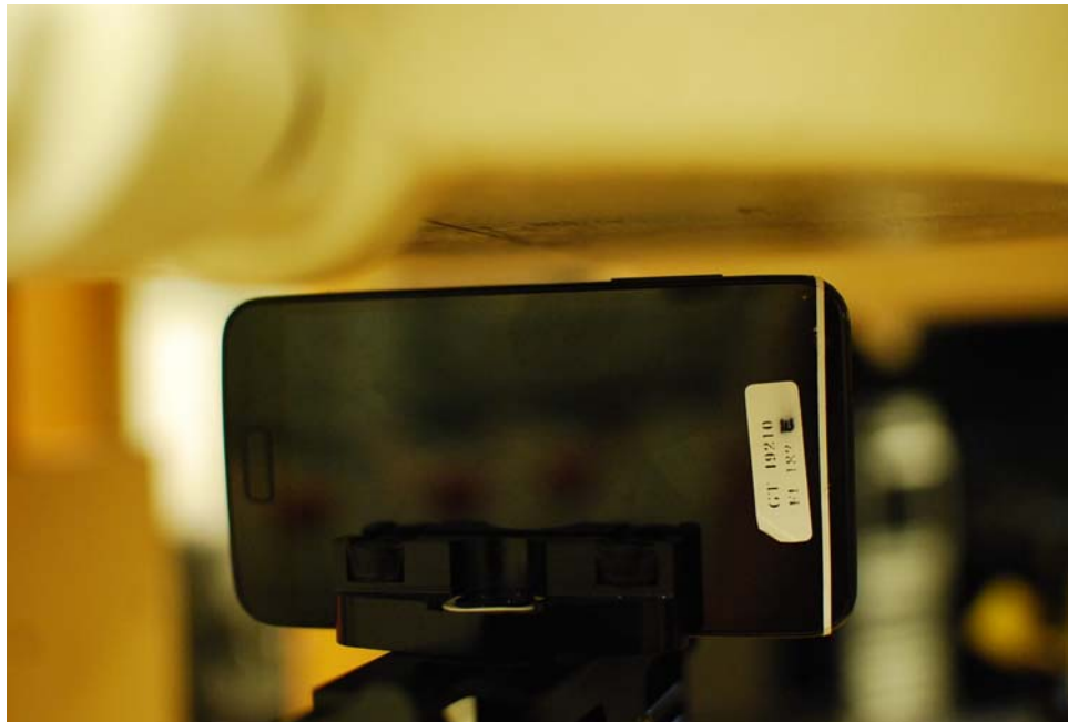
SAR Test Setup Photo 10: Left at 1.0 cm
