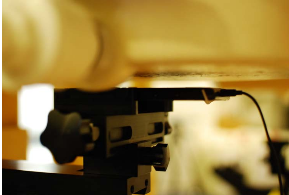
SAR Test Setup Photo 11: Body-Worn at 1.0 cm
