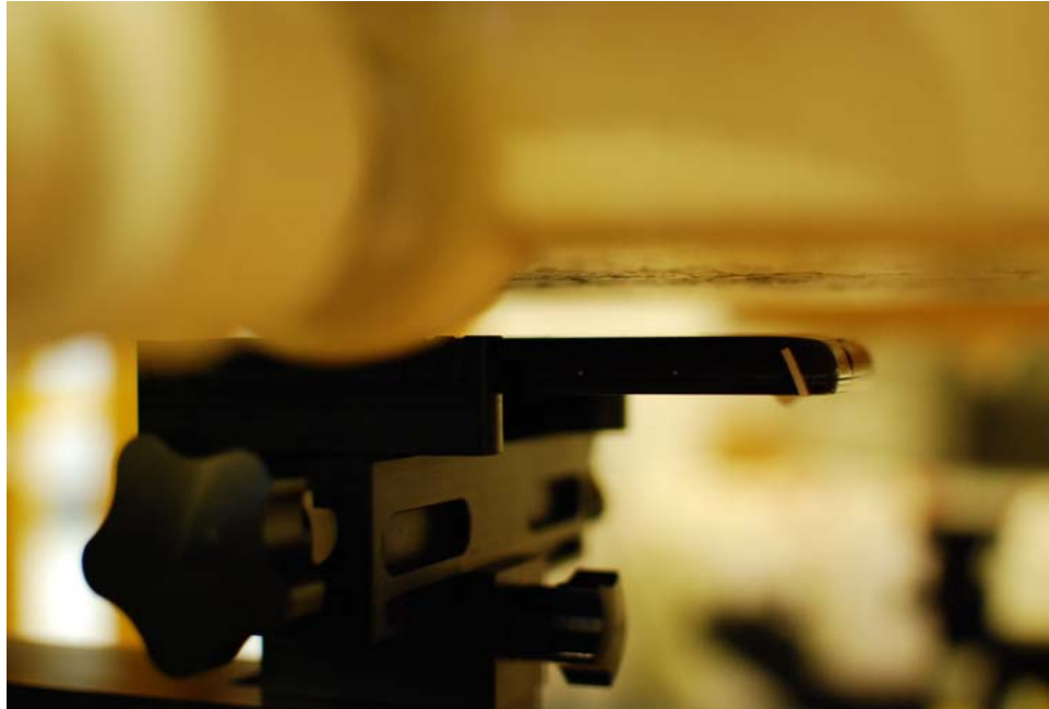
SAR Test Setup Photo 5: Back at 1.0 cm
