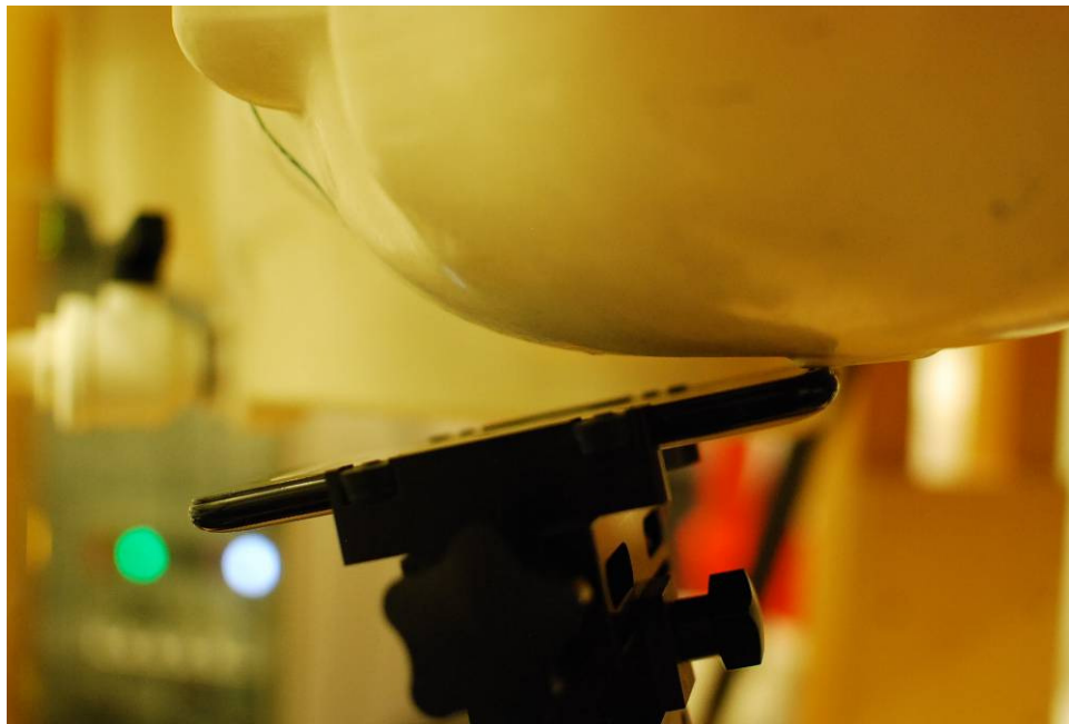
SAR Test Setup Photo 4 – Left Tilt
