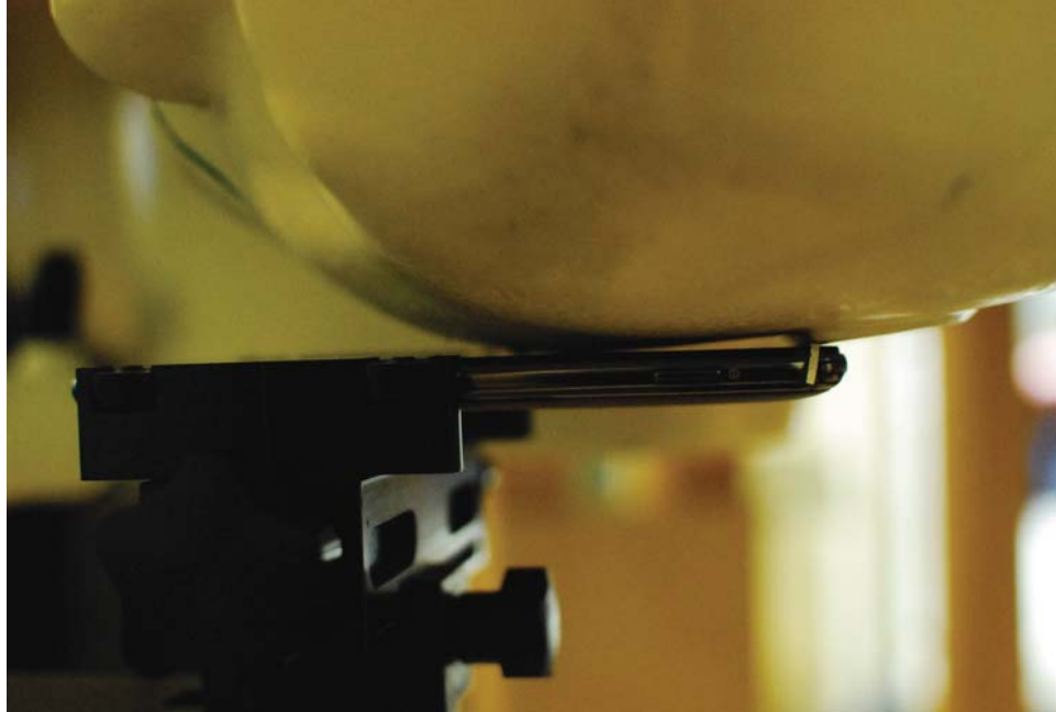
SAR Test Setup Photo 3: Left Touch
