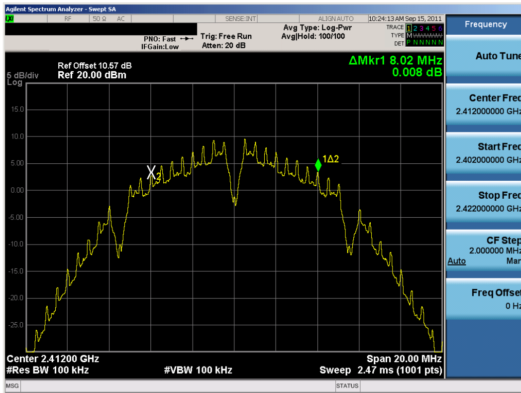
Plot 6-1. 6dB Bandwidth Plot (802.11b – Ch. 1)
