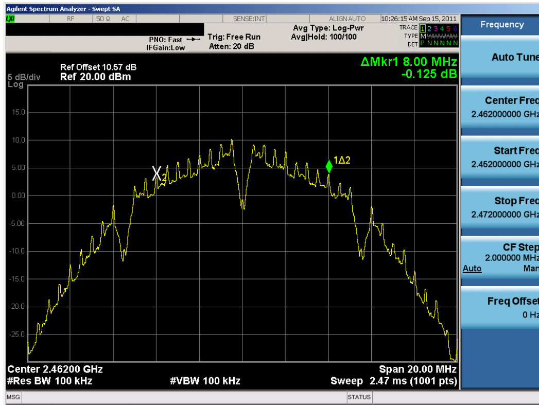
Plot 6-3. 6dB Bandwidth Plot (802.11b – Ch. 11)
