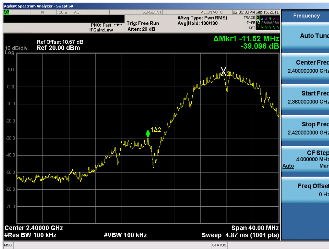
Plot 6-31. Band Edge Plot (802.11b – Ch. 1)
