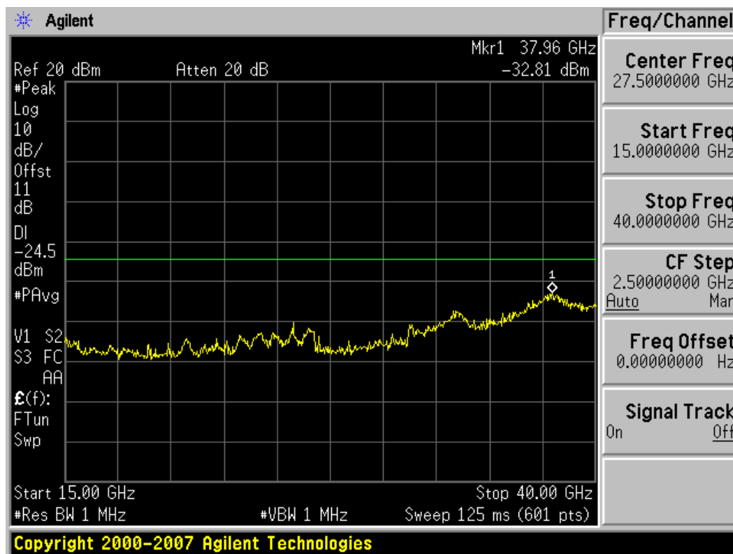
Plot 6-48. Conducted Spurious Plot (802.11a – Ch. 149)
