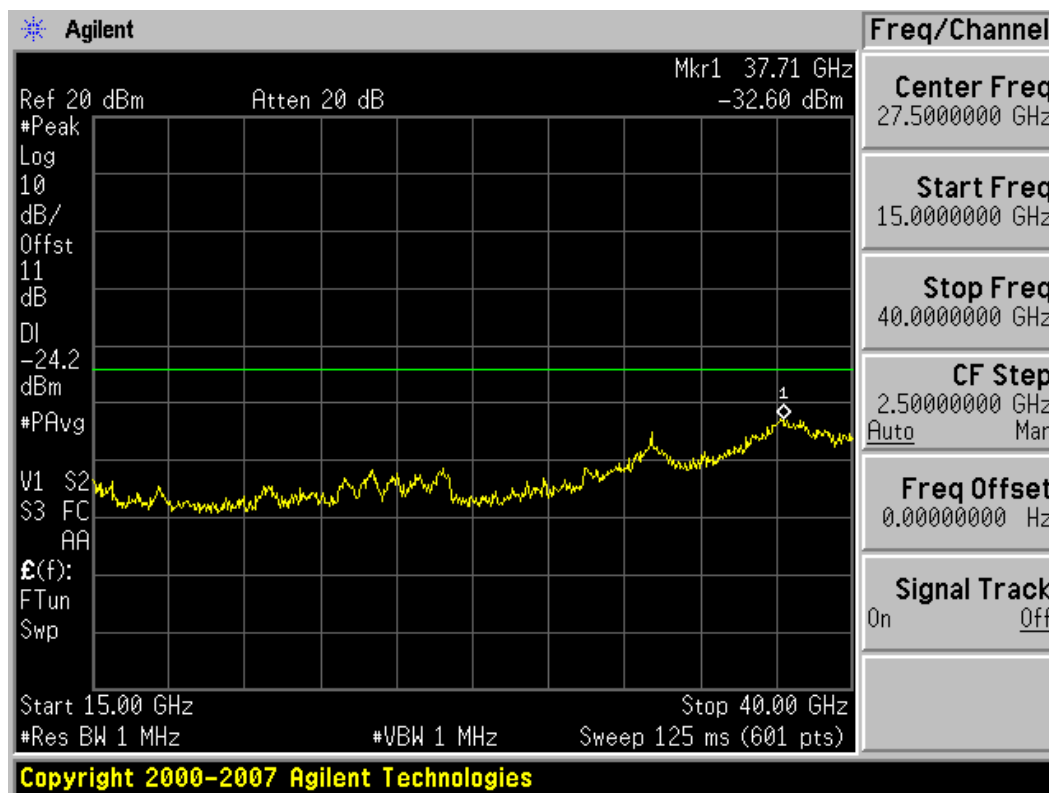
Plot 6-50. Conducted Spurious Plot (802.11a – Ch. 157)
