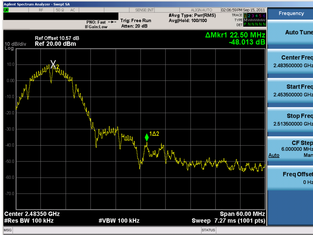
Plot 6-32. Band Edge Plot (802.11b – Ch. 11)
