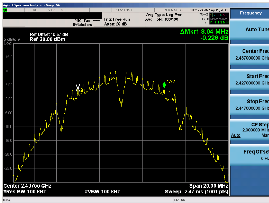
Plot 6-2. 6dB Bandwidth Plot (802.11b – Ch. 6)
