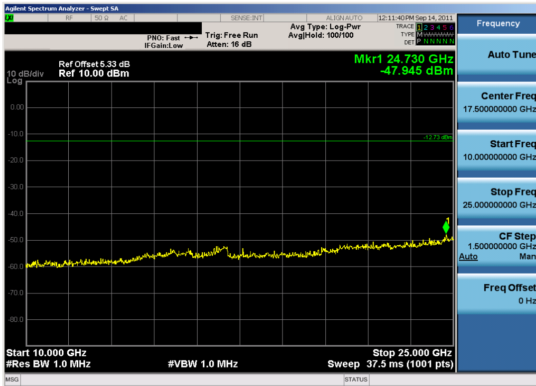
Plot 6-21. Conducted Spurious Plot (Bluetooth, 1Mbps – Ch. 39)
