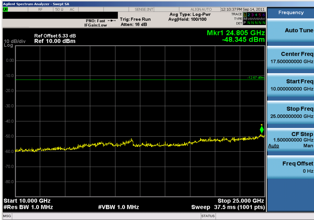
Plot 6-19. Conducted Spurious Plot (Bluetooth, 1Mbps – Ch. 0)
