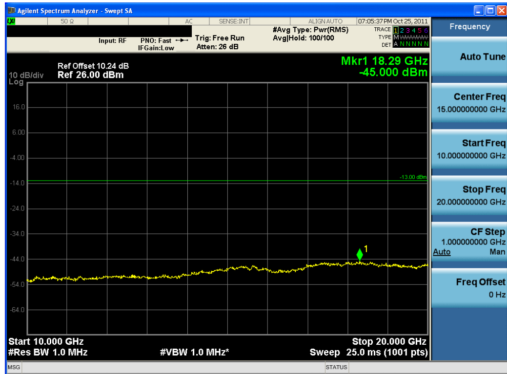
Plot 7-10. Conducted Spurious Plot (AWS WCDMA Mode – Ch. 1862)
