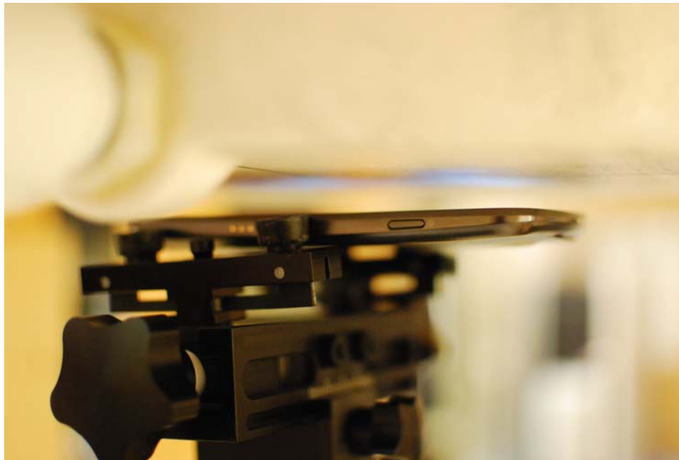
SAR Test Setup Photo 6: Front at 1.0 cm
