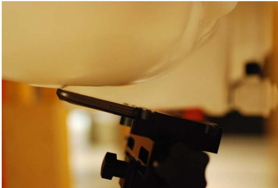
SAR Test Setup Photo 2: Right Tilt
