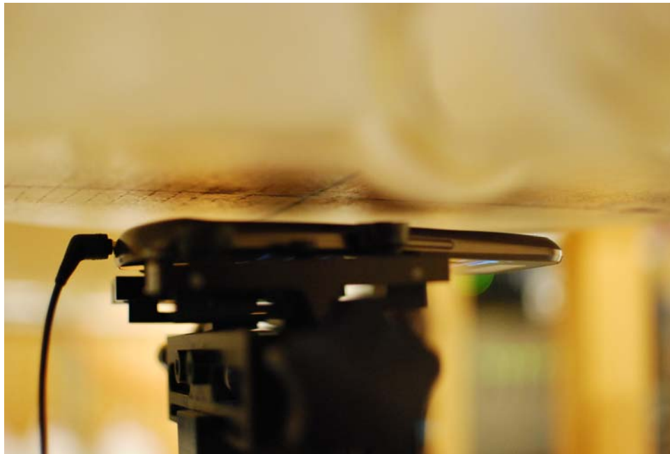
SAR Test Setup Photo 10: Body-Worn at 1.0 cm
