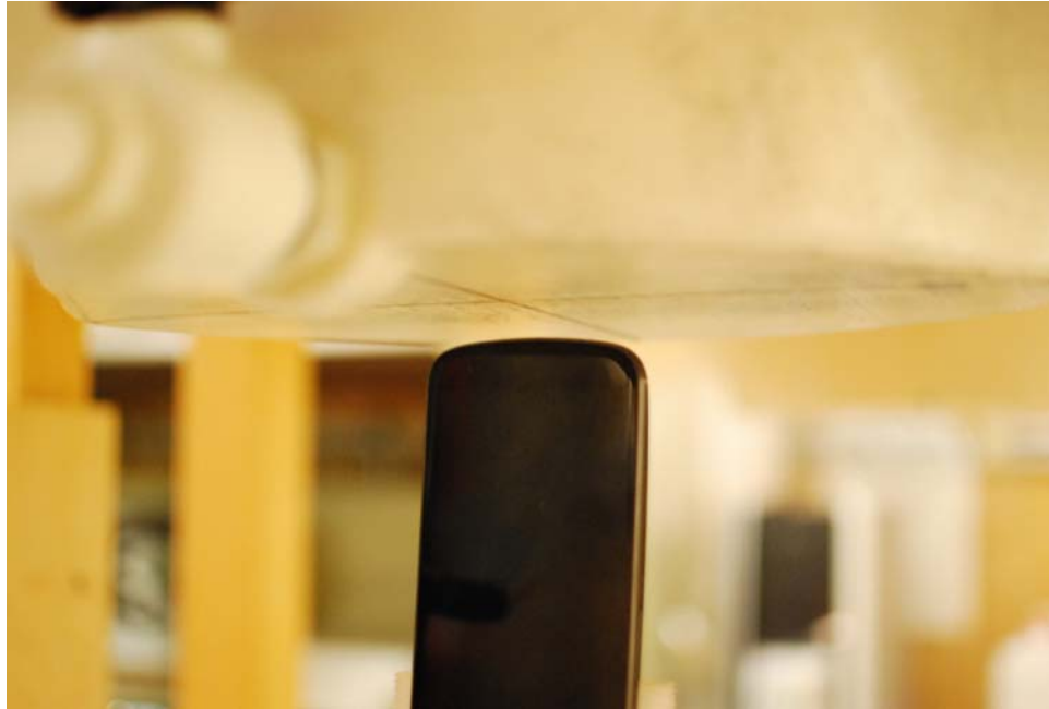
SAR Test Setup Photo 7: Bottom at 1.0 cm
