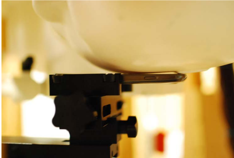
SAR Test Setup Photo 3: Left Touch
