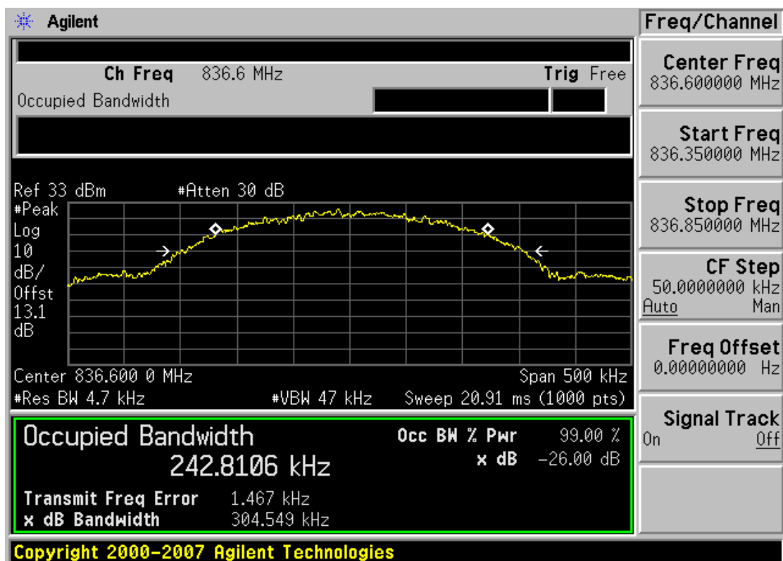
Plot 7-10. Occupied Bandwidth Plot (EDGE850 Mode – Ch. 190)
