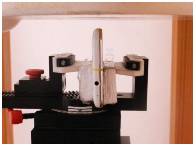
Right Side with Phantom 1 cm Gap
