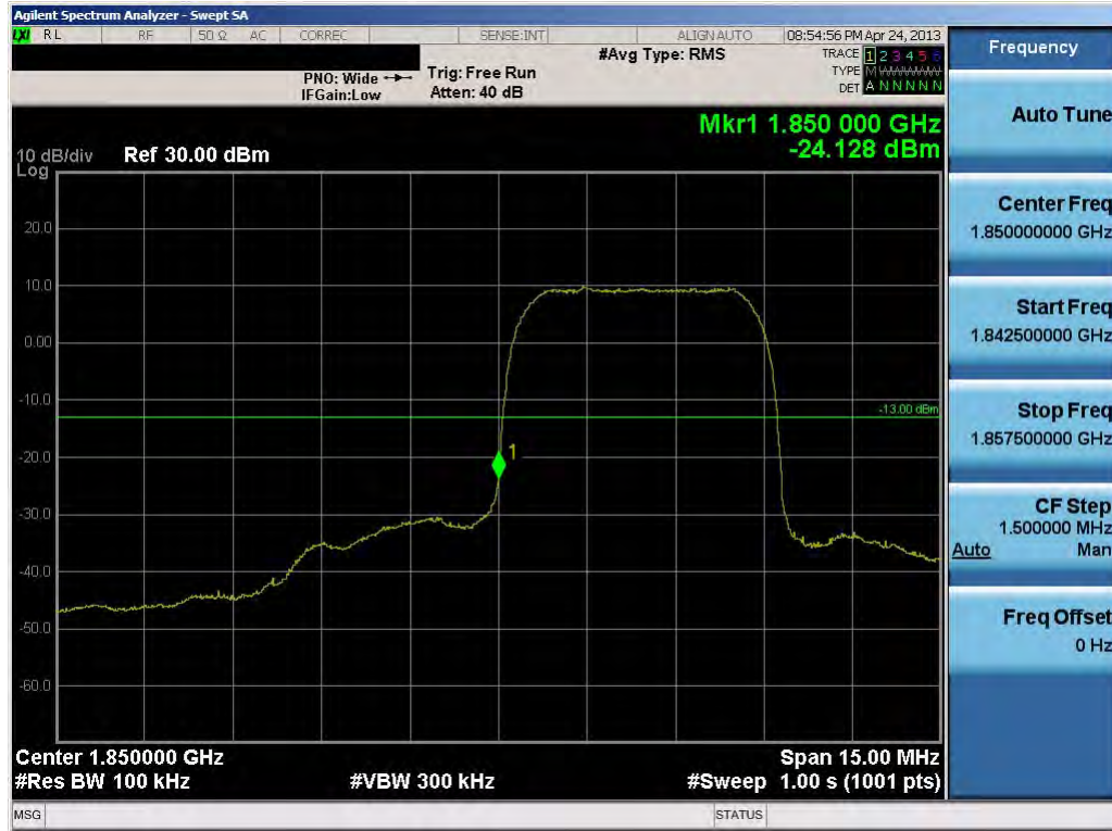
Plot 7-37. Band Edge Plot (PCS WCDMA Mode – Ch. 9262)
