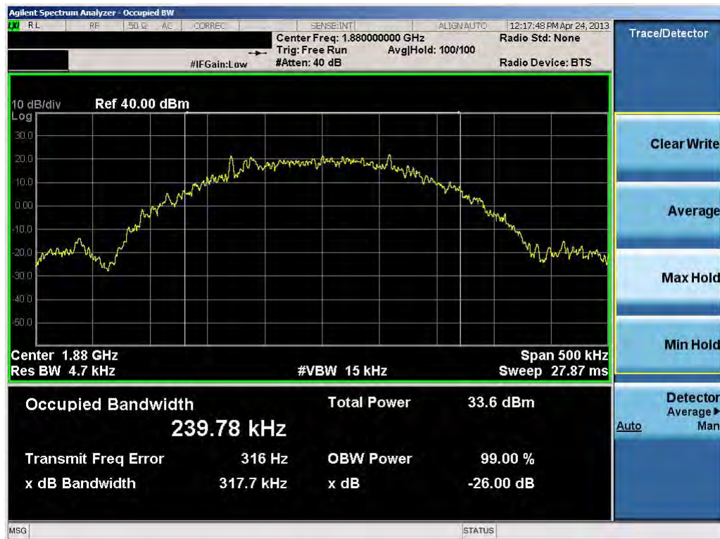
Plot 7-24. Occupied Bandwidth Plot (EDGE1900 Mode – Ch. 661)
