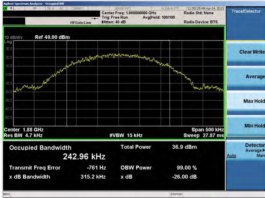
Plot 7-19. Occupied Bandwidth Plot (PCS GSM Mode – Ch. 661)
