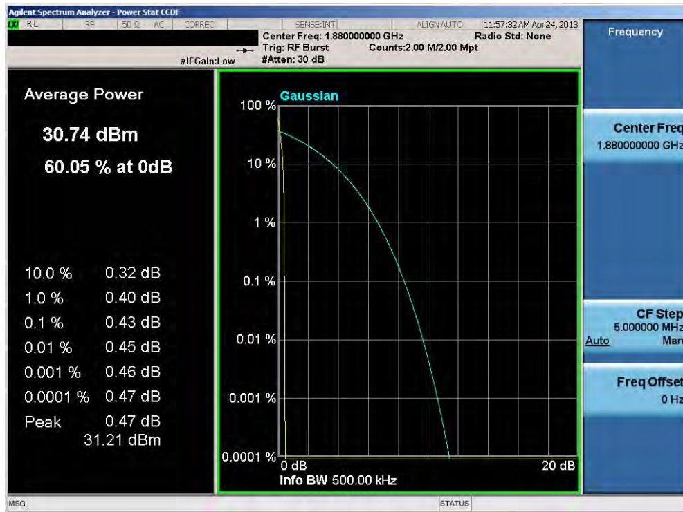
Plot 7-20. Peak-Average Ratio Plot (PCS GSM Mode – Ch. 661)
