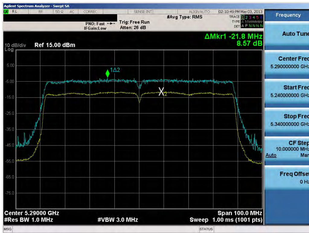
Plot 6-60. Peak Excursion Ratio Plot (80MHz BW 802.11ac)
