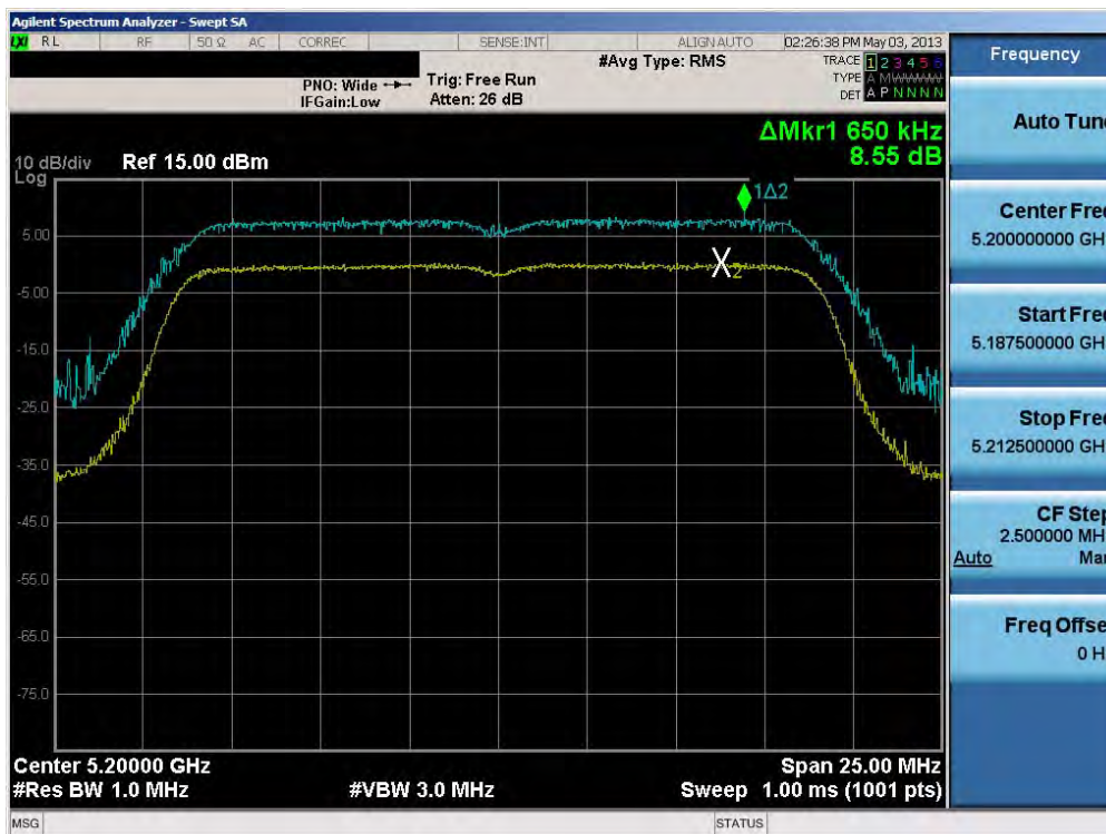
Plot 6-58. Peak Excursion Ratio Plot (20MHz BW 802.11n)
