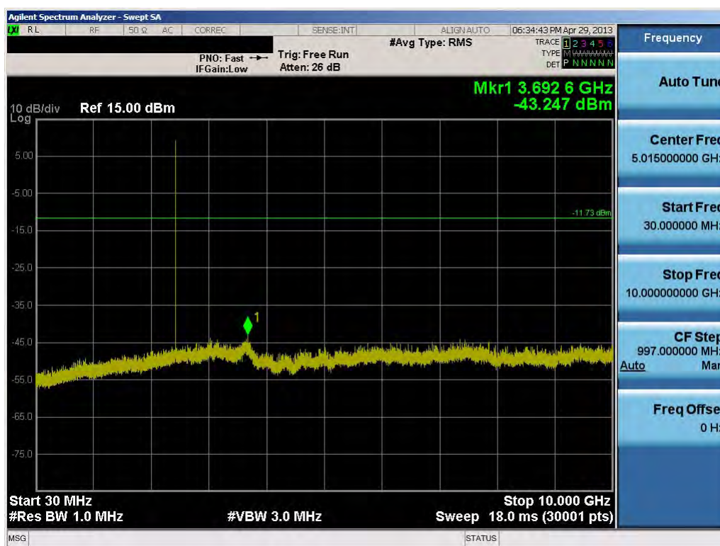
Plot 6-38. Conducted Spurious Plot (Bluetooth, 1Mbps – Ch. 39)
