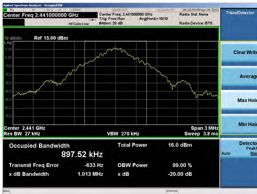
Plot 6-2. 20dB Bandwidth Plot (Bluetooth, 1Mbps – Ch. 39)
