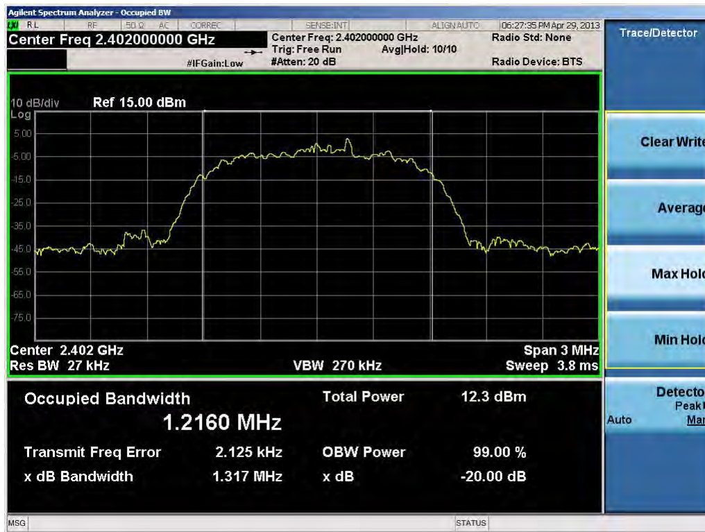
Plot 6-7. 20dB Bandwidth Plot (Bluetooth, 3Mbps – Ch. 0)
