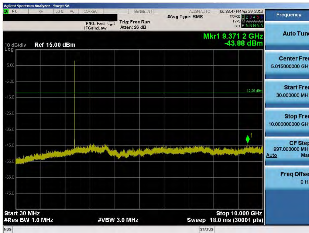
Plot 6-36. Conducted Spurious Plot (Bluetooth, 1Mbps – Ch. 0)
