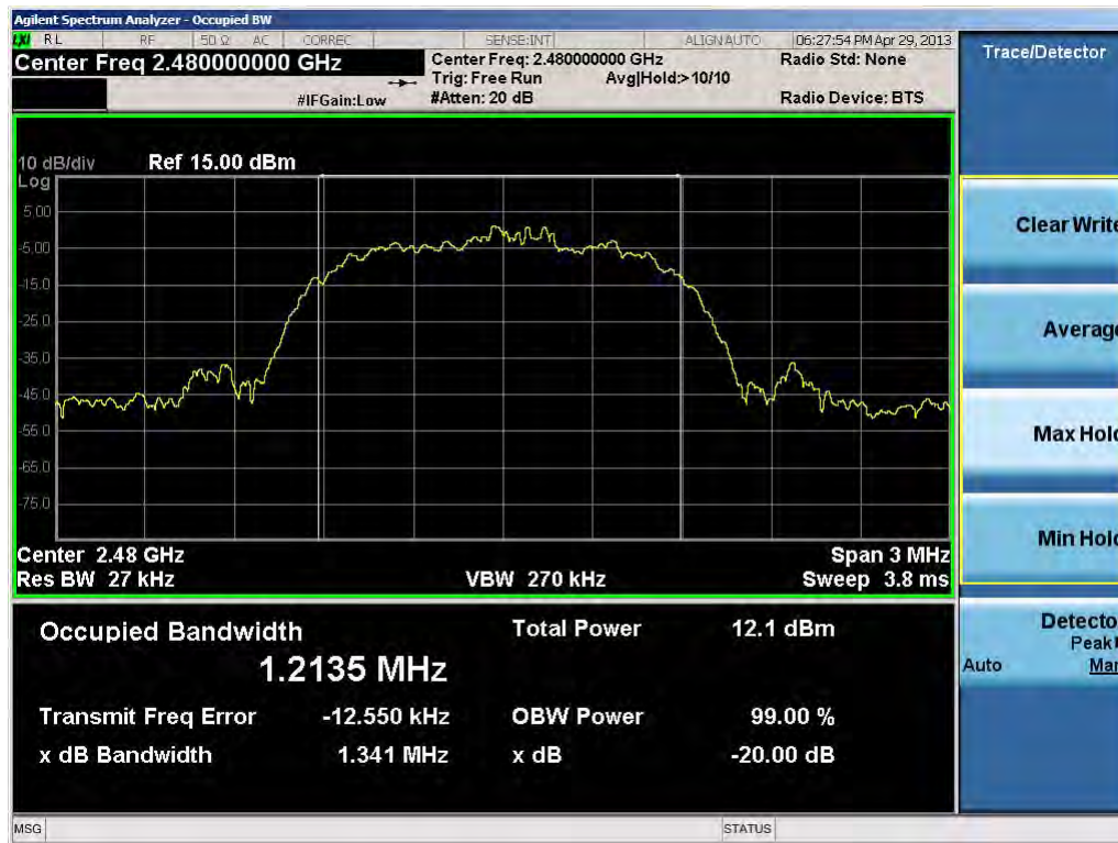
Plot 6-9. 20dB Bandwidth Plot (Bluetooth, 3Mbps – Ch. 78)
