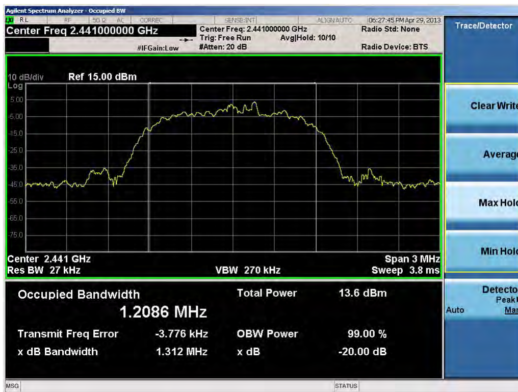
Plot 6-8. 20dB Bandwidth Plot (Bluetooth, 3Mbps – Ch. 39)
