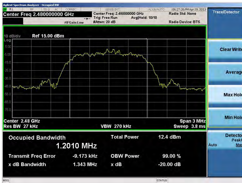
Plot 6-6. 20dB Bandwidth Plot (Bluetooth, 2Mbps – Ch. 78)
