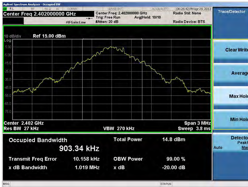
Plot 6-1. 20dB Bandwidth Plot (Bluetooth, 1Mbps – Ch. 0)
