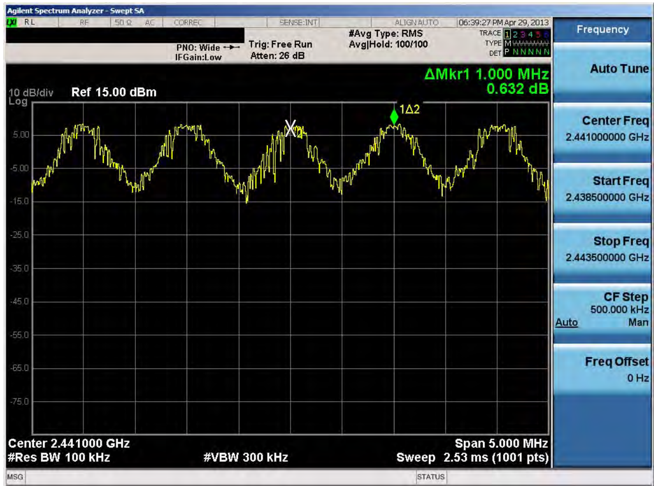
Plot 6-32. Channel Spacing Plot (Bluetooth)
