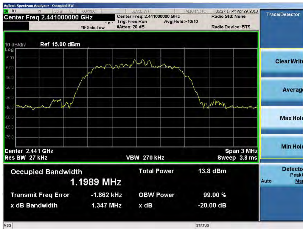
Plot 6-5. 20dB Bandwidth Plot (Bluetooth, 2Mbps – Ch. 39)
