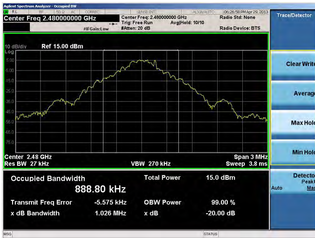
Plot 6-3. 20dB Bandwidth Plot (Bluetooth, 1Mbps – Ch. 78)
