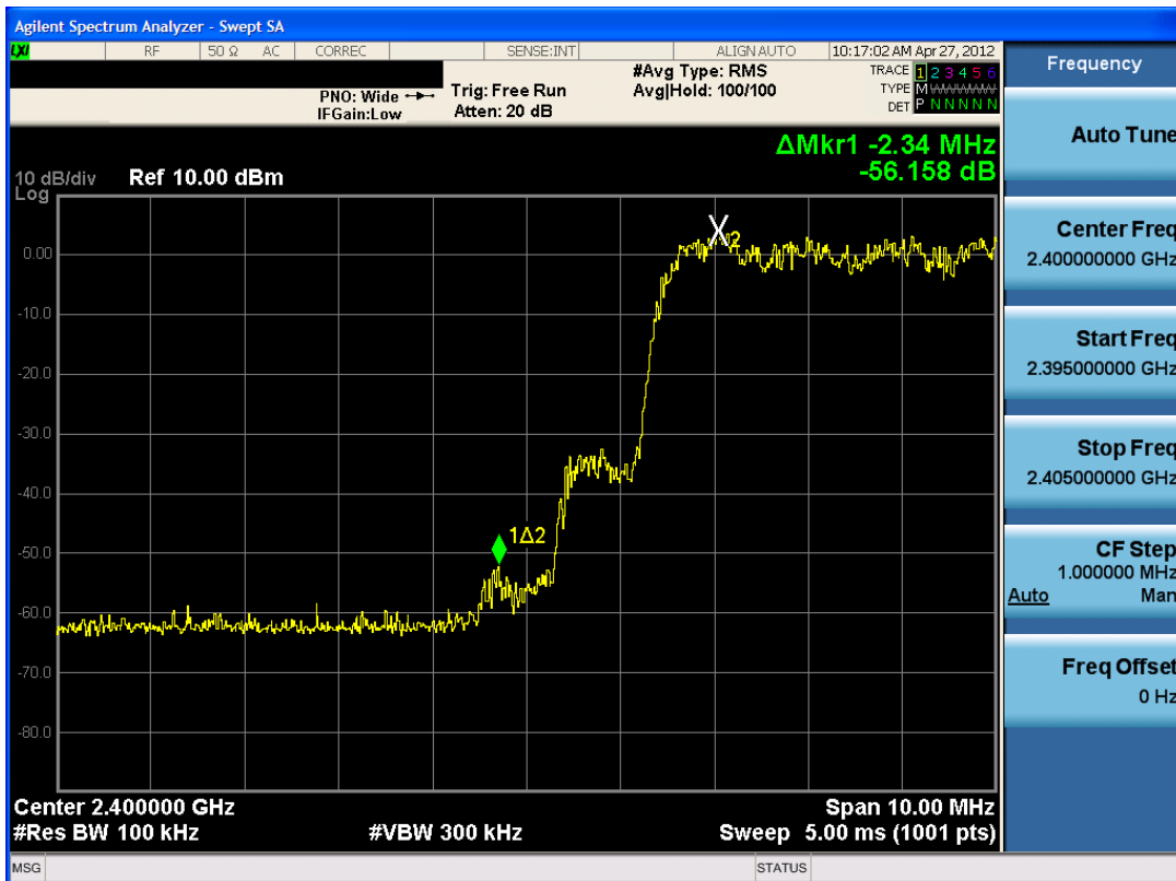
Plot 6-12. Band Edge Plot (Bluetooth with Hopping Enabled, 1Mbps – Ch. 0)
