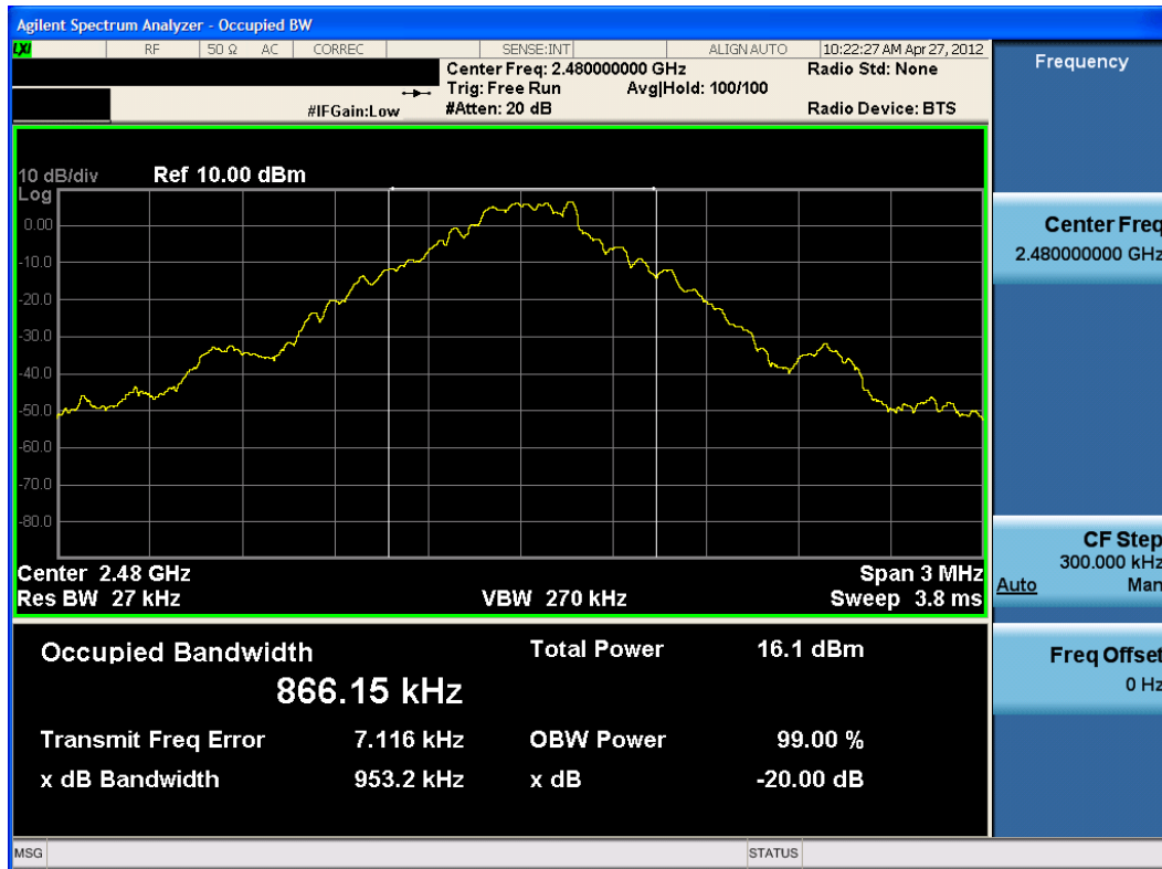
Plot 6-3. 20dB Bandwidth Plot (Bluetooth, 1Mbps – Ch. 78)
