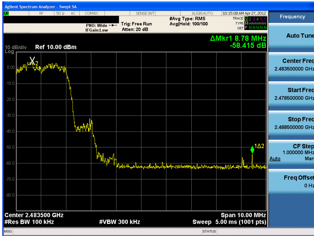
Plot 6-13. Band Edge Plot (Bluetooth with Hopping Enabled, 1Mbps – Ch. 78)
