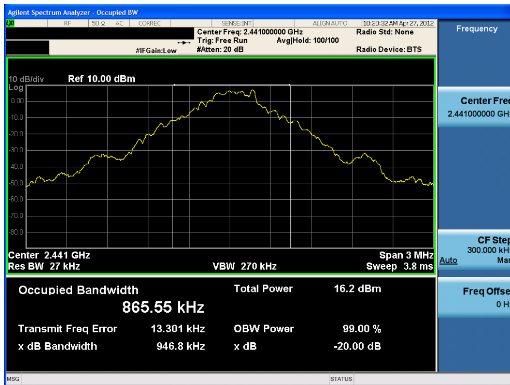
Plot 6-2. 20dB Bandwidth Plot (Bluetooth, 1Mbps – Ch. 39)
