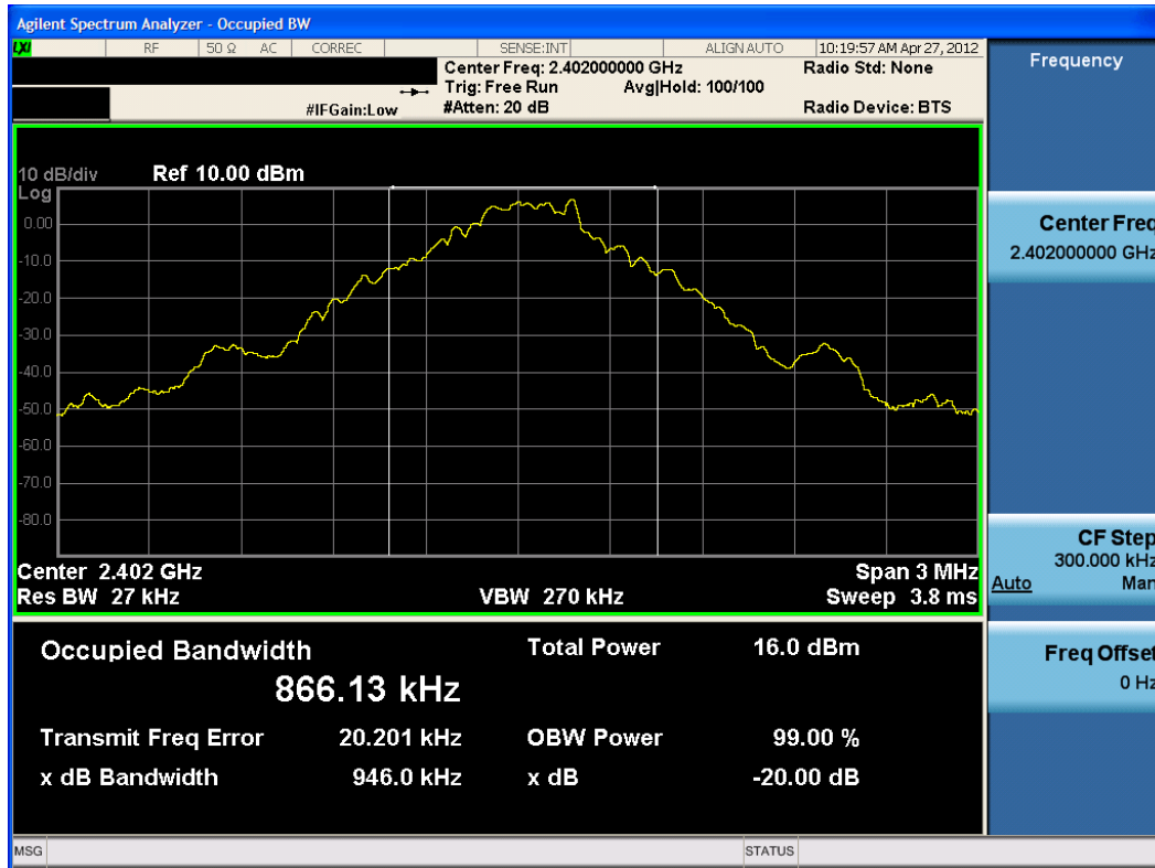
Plot 6-1. 20dB Bandwidth Plot (Bluetooth, 1Mbps – Ch. 0)
